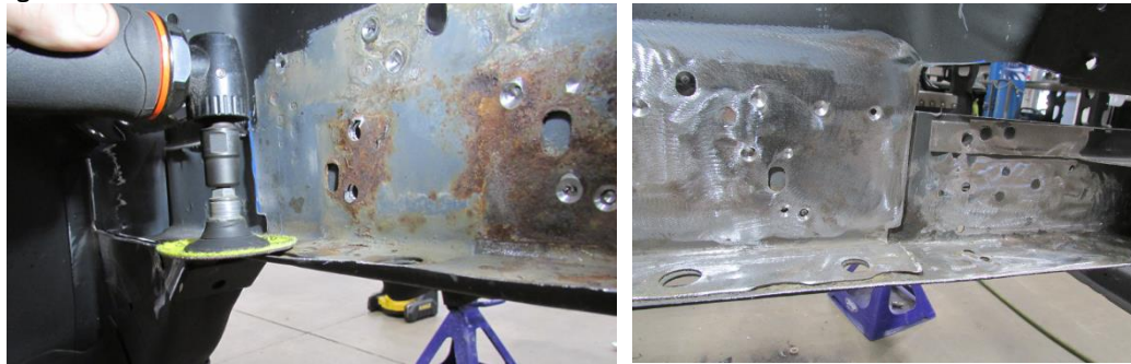
Figure 14 - Clean up cut edges
