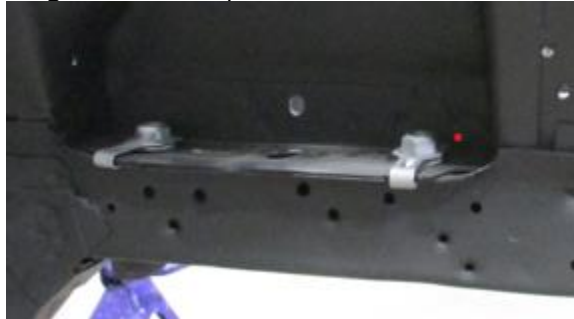
Figure 2 - K Member Mounting Hardware
