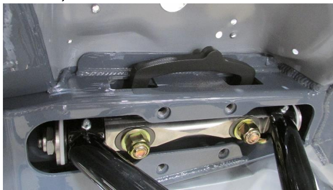
Figure 25 - Install Upper Control Arm
