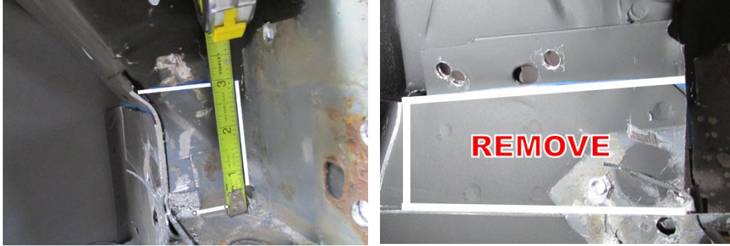
Figure 13 - Remove rear outer rail and strut tower material
