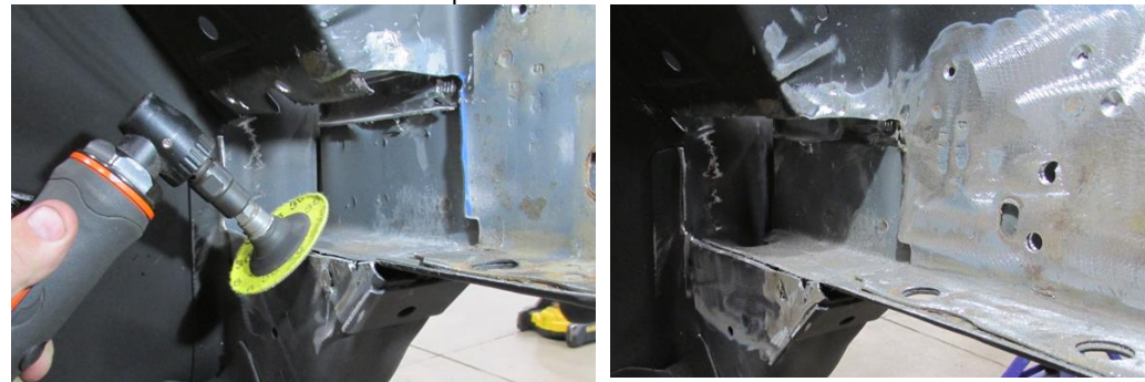
Figure 15 - Prepare sheet metal
