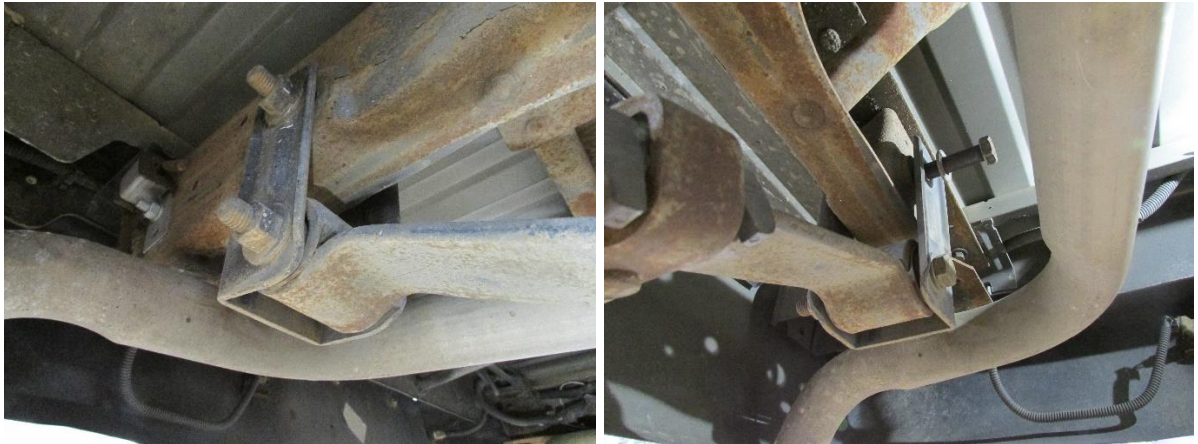
Figure 1 - Remove Factory Leaf Spring Shackle
