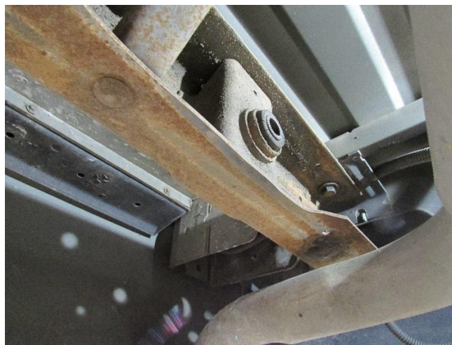
Figure 2 - Remove Factory Leaf Spring Bushing
