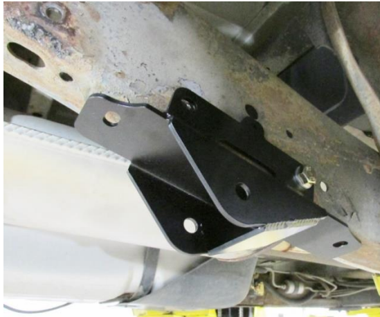
Figure 4 - Install Front Mounts
