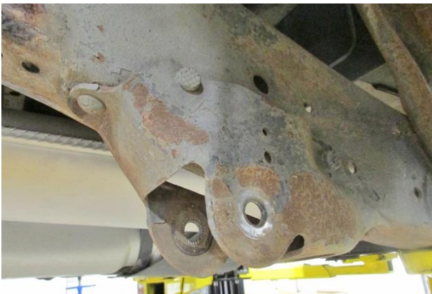
Figure 3 - Remove Front Mounts
