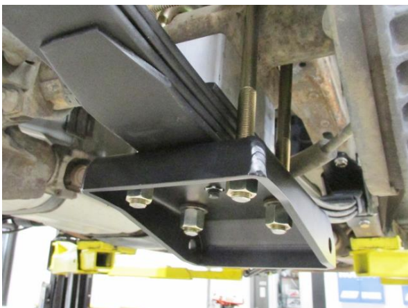
Figure 6 - Install Spring Plates
