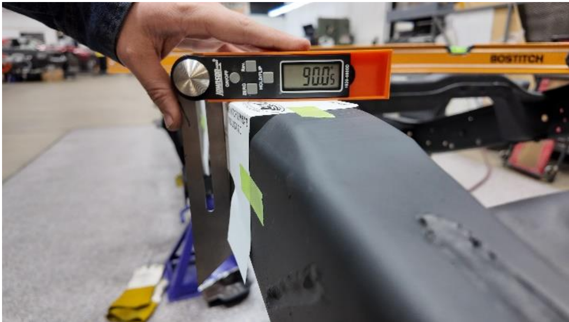
Figure 10 – Fold Notch Template and Place on Frame at 90 Degrees
