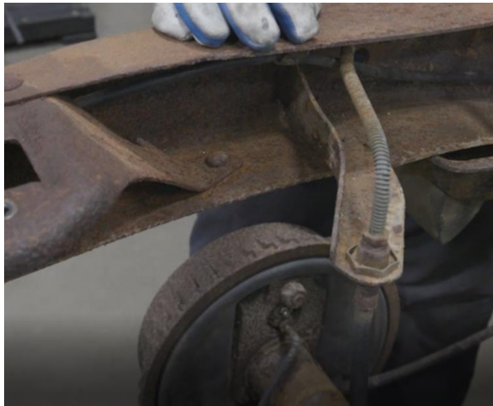
Figure 2 - Disconnect Factory Rear Brake Hose
