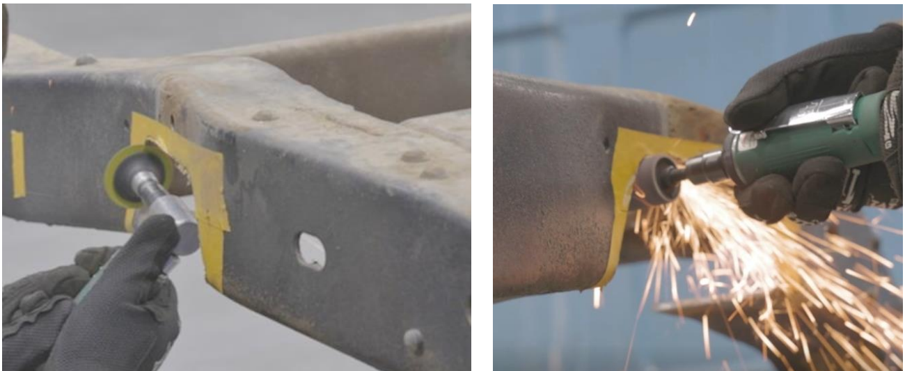
Figure 13 - Grind Notch Area
