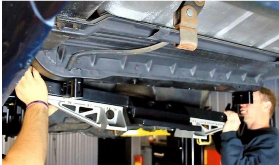
Figure 83 - Install Upper Cradle Assembly to Frame
