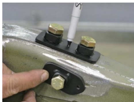
Figure 46 – Framerail Nut Plate Location
