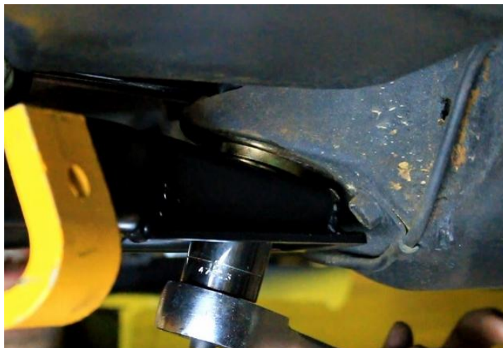
Figure 90 - Torque Lower Differential Mount
