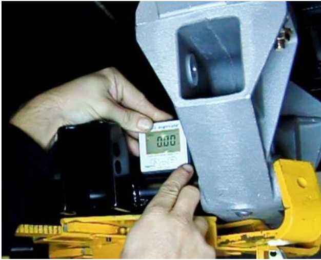
Figure 42 - Level IRS Cradle to the Frame
