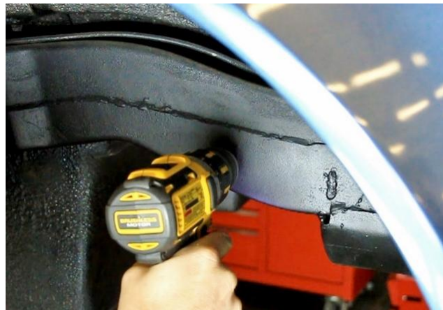
Figure 54 – Drill through Frame Rail
