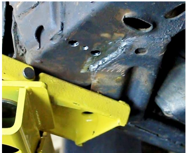
Figure 29 – Trailing Link Bracket Nut Plate
