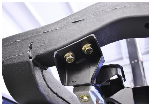
Figure 80 - Install Upper Cradle Assembly to Frame
