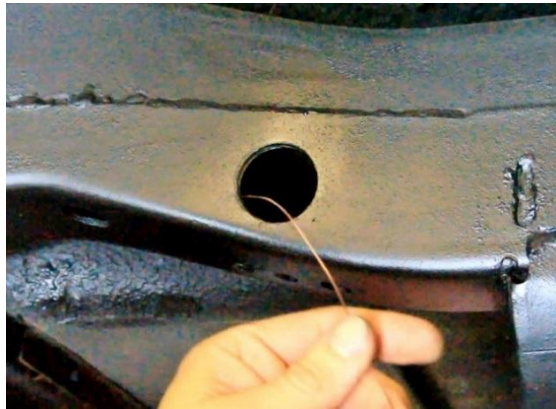
Figure 59 – Locate Lower Cradle Nut Plate
