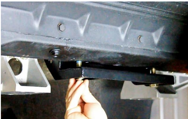
Figure 84 - Install Fasteners & Slotted Shims
