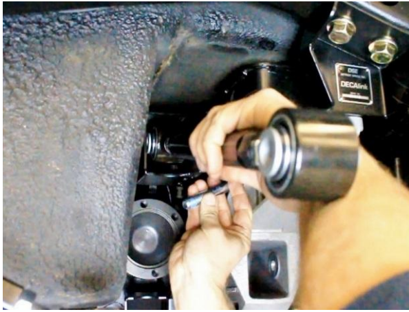
Figure 97 – Install Upper Lateral Link & Tie Braces
