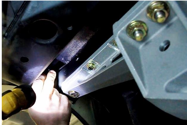
Figure 50 - Scribe Inside Mounting Hole Location
