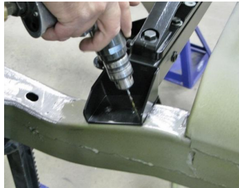
Figure 45 – Drill IRS Cradle Mount Locations
