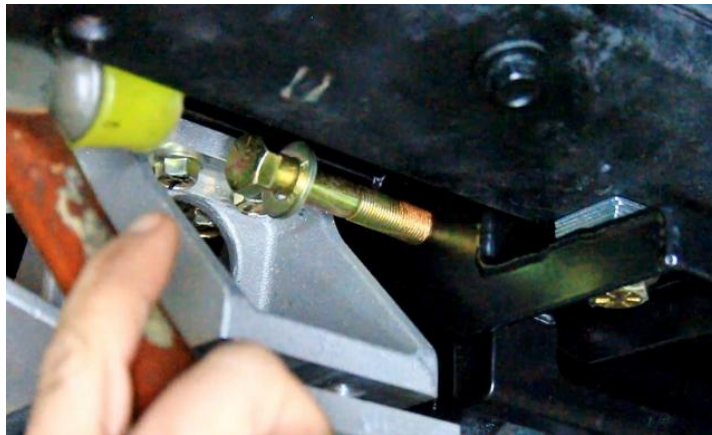
Figure 89 - Install Differential to Upper Cradle
