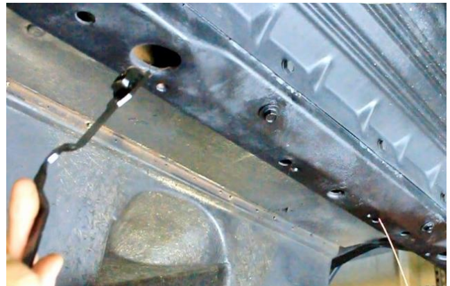
Figure 36 - Bend Crossmember Nut Plate
