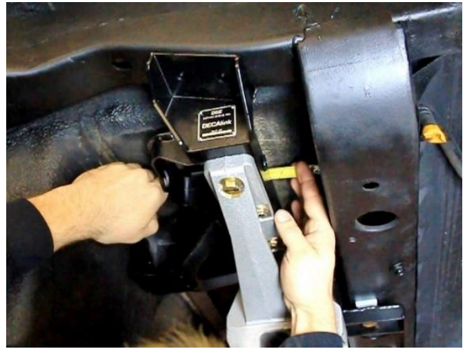
Figure 42 - Level IRS Cradle to the Frame
