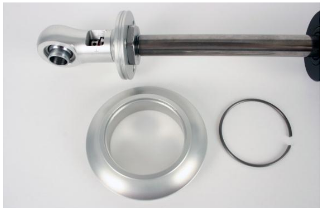
Figure 109 - Spring Seat & Retaining Ring
