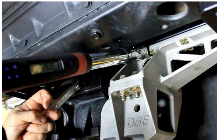
Figure 92 - Torque Upper Differential Bracket
