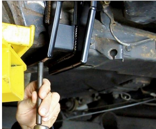
Figure 25 - Transfer Punch & Drill the Frame
