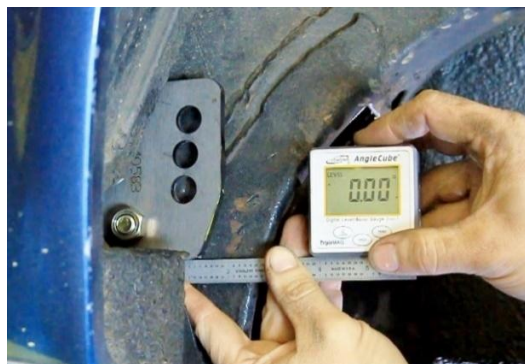
Figure 8 - Level Frame Doubler Plates
