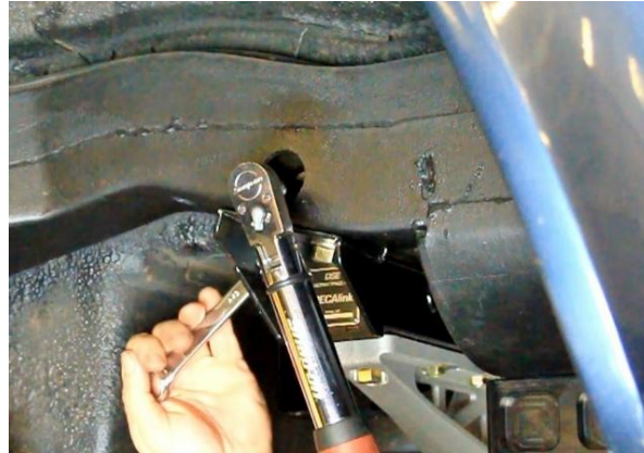
Figure 86 – Torque Inner Frame Rail Fasteners
