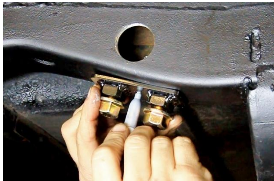
Figure 57 – Framerrail Nut Plate Location
