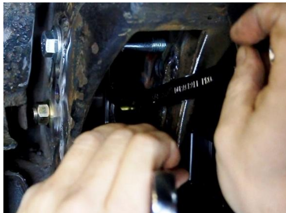
Figure 24 - Expand Crush Sleeve
