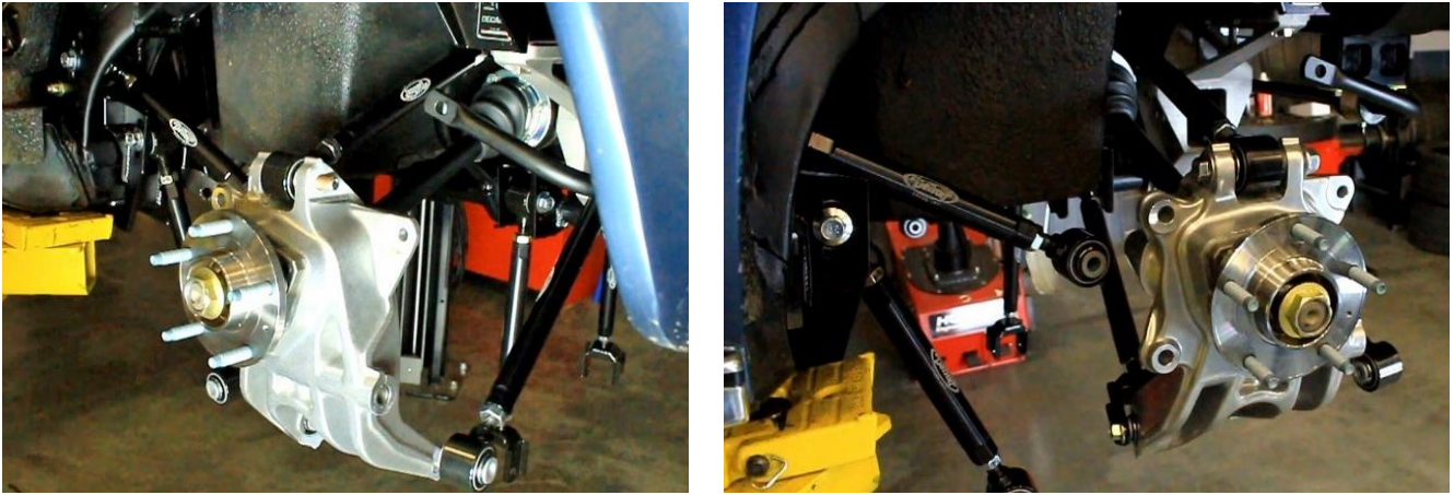
Figure 104 - Attach Lateral Links to Upright
