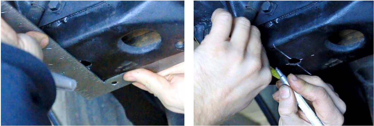
Figure 61 - Sway Bar Nut Plate Location
