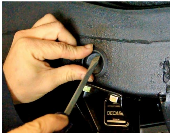
Figure 114 – Install Recessed Plug
