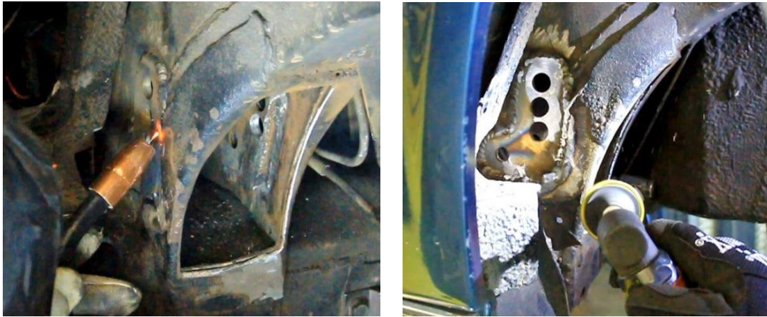
Figure 22 - Finish Weld Doubler Plates
