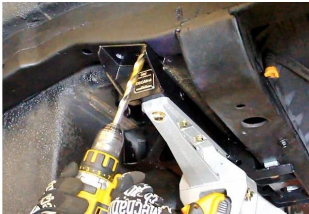
Figure 51 - Drill Bottom Side of Frame
