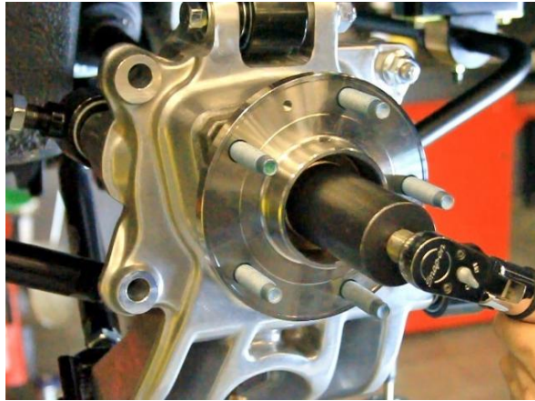
Figure 113 – Torque Outer CV Joint
