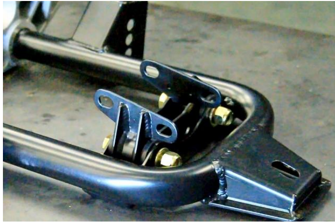
Figure 78 - Lower Differential Bracket Assembly
