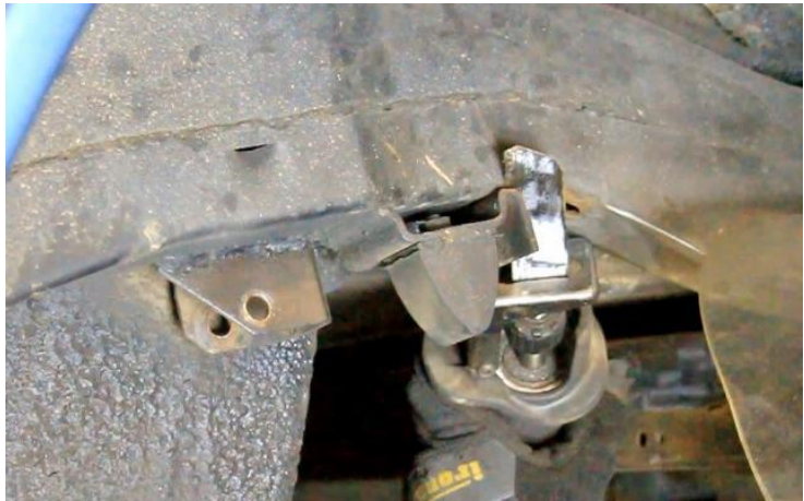
Figure 4 – Remove Frame Bumper and Upper Shock Mount Brackets
