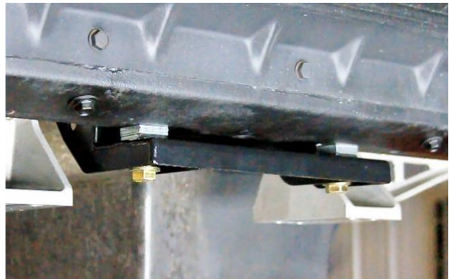
Figure 84 - Install Fasteners & Slotted Shims
