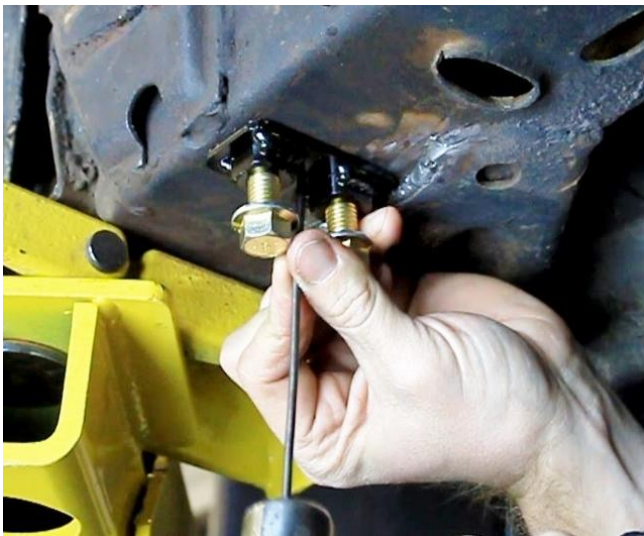
Figure 29 – Trailing Link Bracket Nut Plate
