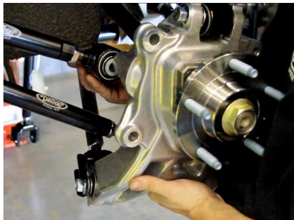
Figure 105 - Install Upper & Lower Trailing Links
