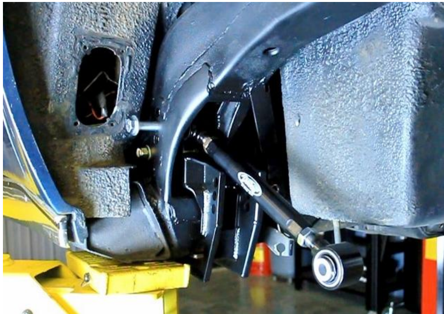
Figure 94 – Install the IRS Lower Trailing Links
