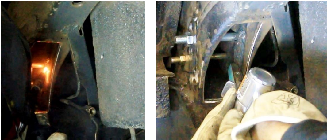
Figure 20 – Weld Inner Frame Rail
