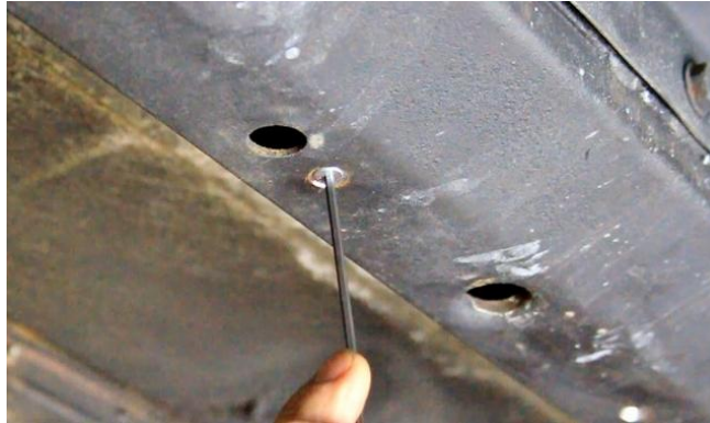
Figure 35 - Drill & Chamfer Holes
