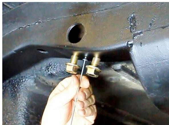
Figure 60 – Install Nut Plate Assemblies
