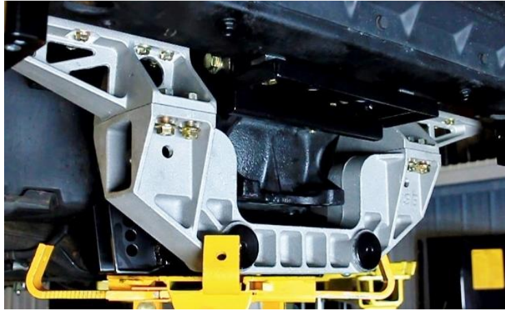
Figure 91 - Assemble the IRS Upper and Lower Cradle
