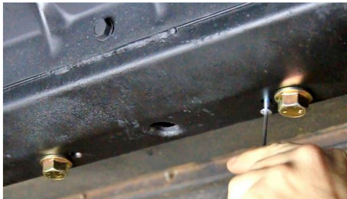
Figure 38 – Install Crossmember Nut Plate
