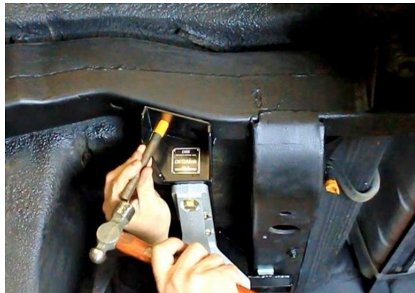
Figure 43 - Transfer Punch Frame for IRS Cradle
