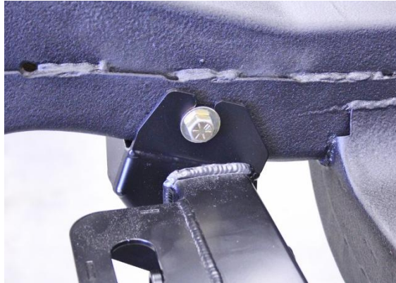
Figure 81 - Install Upper Cradle Assembly to Frame
