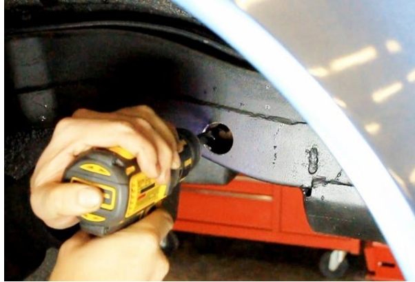
Figure 56 – Drill Inner Mounting Hole
