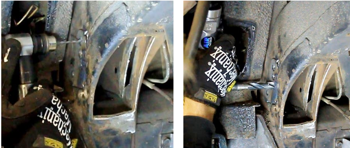
Figure 14 – Drill Trailing Link Holes
