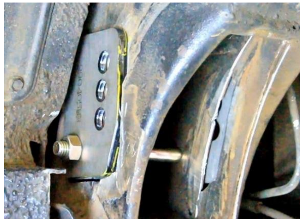
Figure 11 – Verify Frame Rail Modification
