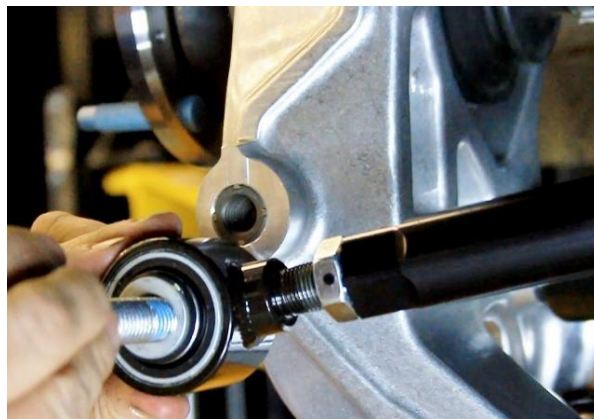
Figure 106 - Install Toe Links
