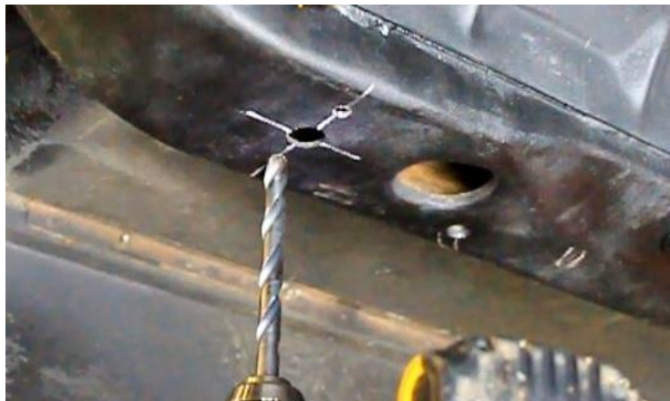
Figure 63 - Drill Sway Bar Nut Plate Location
