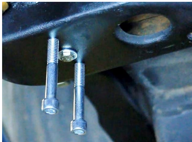
Figure 65 - Install Sway Bracket Nut Plate Assembly
