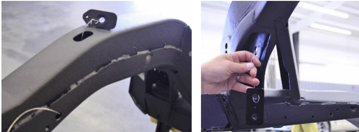
Figure 48 – Position Nut Plate Assemblies
