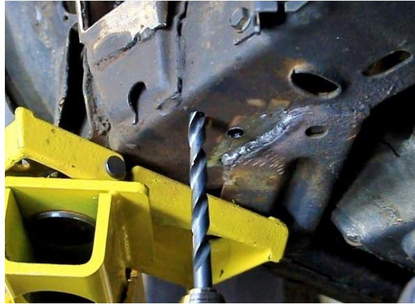
Figure 28 – Drill Trailing Arm Bracket Mounting Locations
