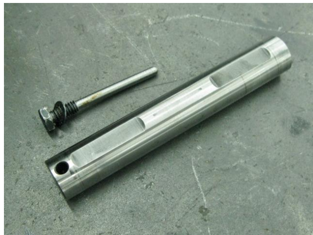
Figure 69 - Cross Shaft & Cross Shaft Bolt Pin
