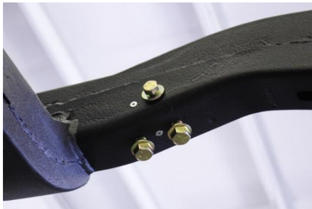
Figure 49 – Install Nut Plate Assemblies
