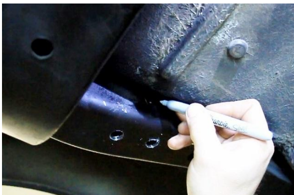
Figure 52 - Locate Inside Mounting Holes
