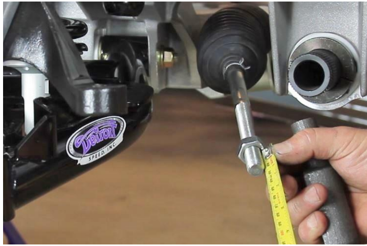
Figure 38 – Install Outer Tie Rods
