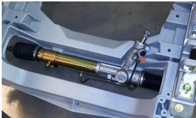
Figure 37 – Installed Rack & Pinion
