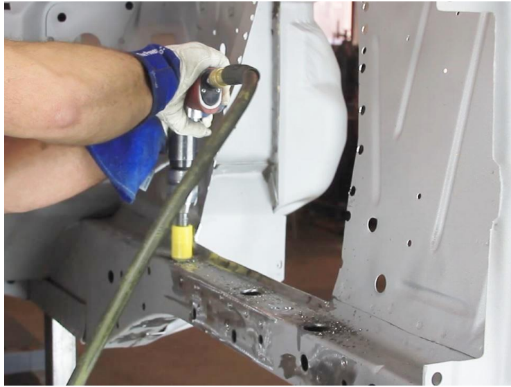
Figure 9 – Drill-Out Top Frameraisls
