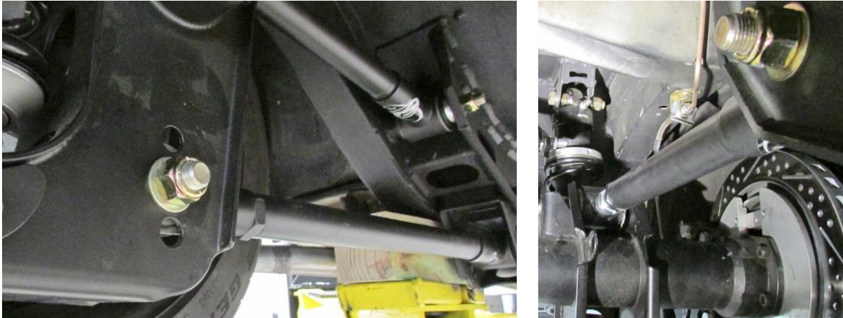
Figure 42 – Install Upper & Lower Links
