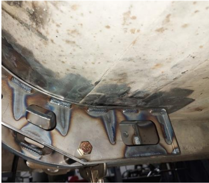
Figure 11 - Locate Torque Box
