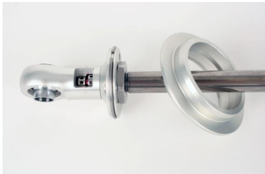
Figure 37 - Removing the Upper Spring Seat
