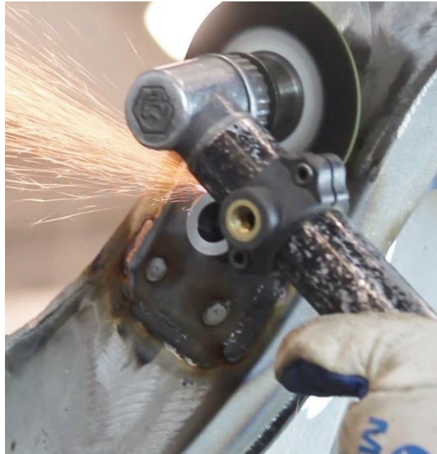
Figure 19 - Cut-Off Crush Tube Flush with Frame Rail
