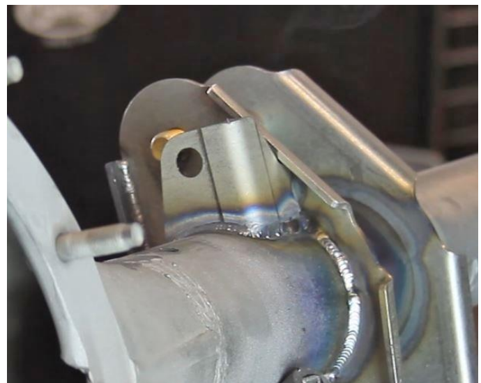
Figure 32 - Weld Sway End-Link Brackets
