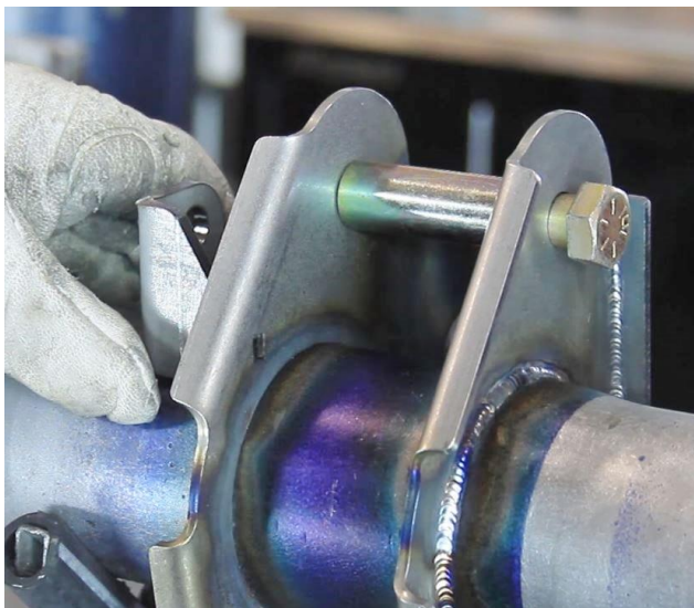
Figure 32 - Weld Sway End-Link Brackets
