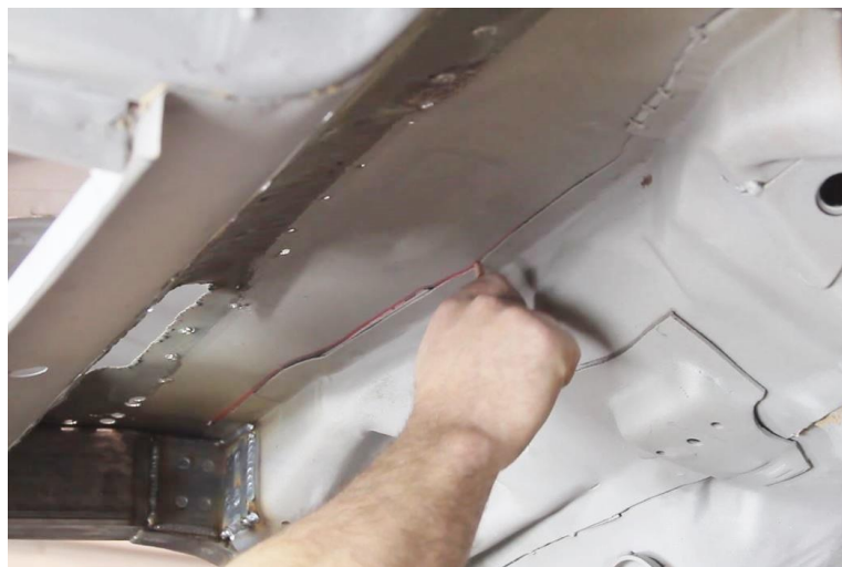
Figure 2 - Mark Floor Pan Cut Line (Underneath Vehicle)
