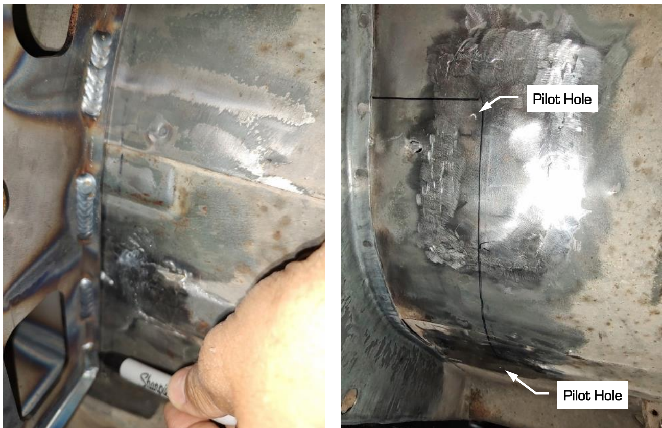
Figure 12 - Trace Torque Box
