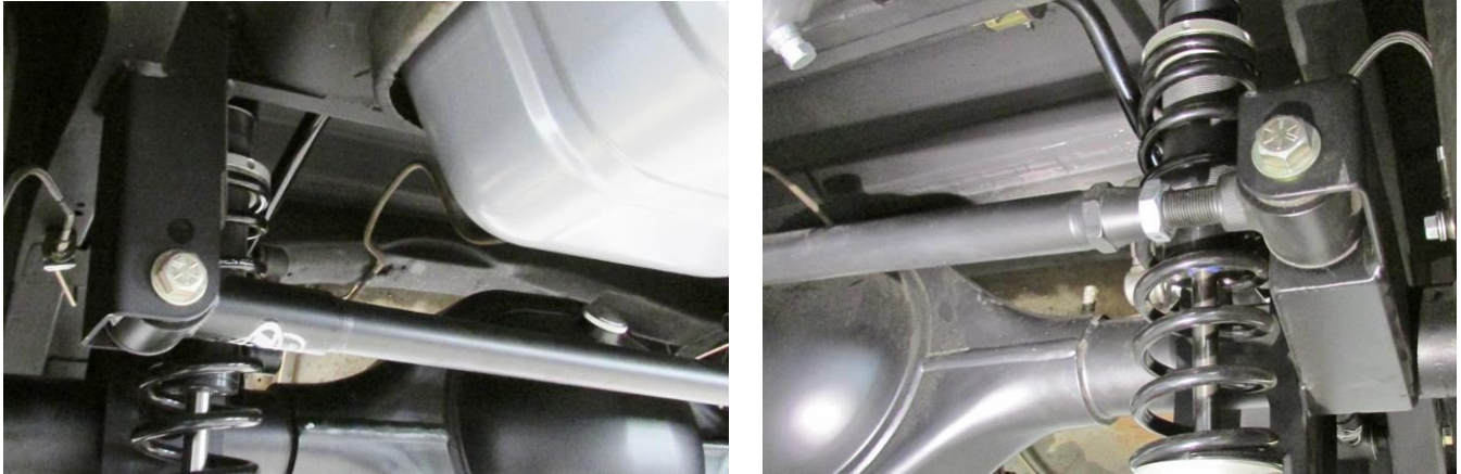
Figure 45 - Install Track Bar
