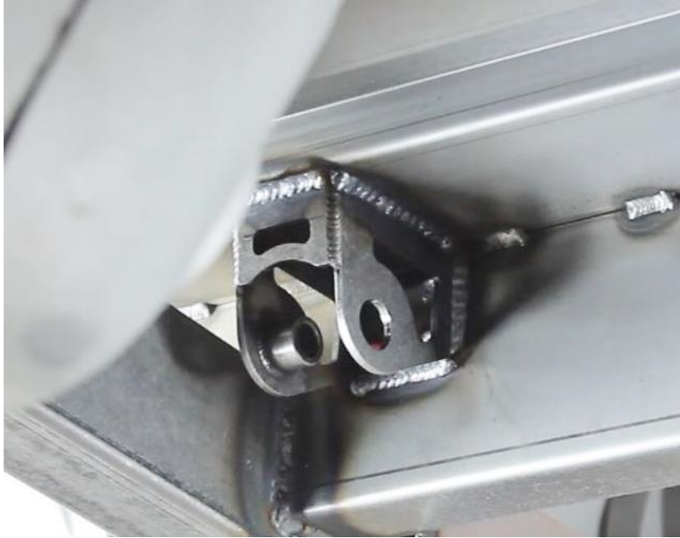
Figure 23 – Weld Upper Shock Mounts
