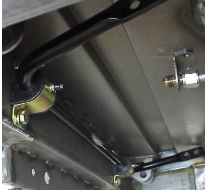
Figure 36 - Install Sway Bar
