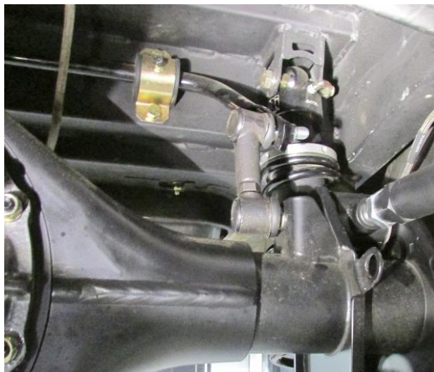
Figure 44 – Attach Sway Bar End-Links
