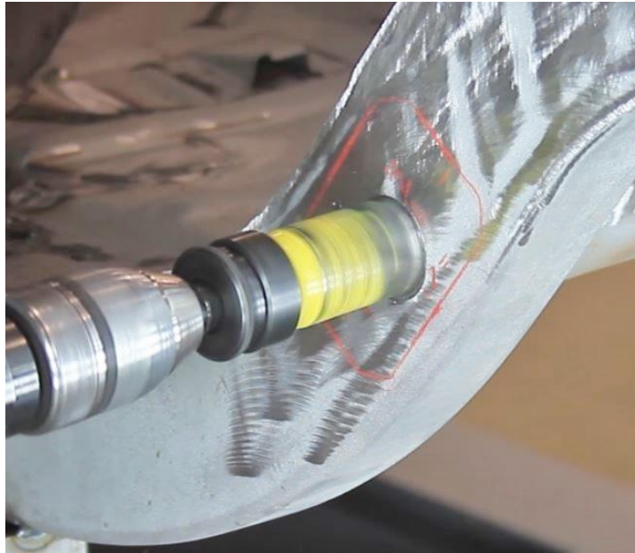
Figure 17 – Drill Upper Link Mount Location
