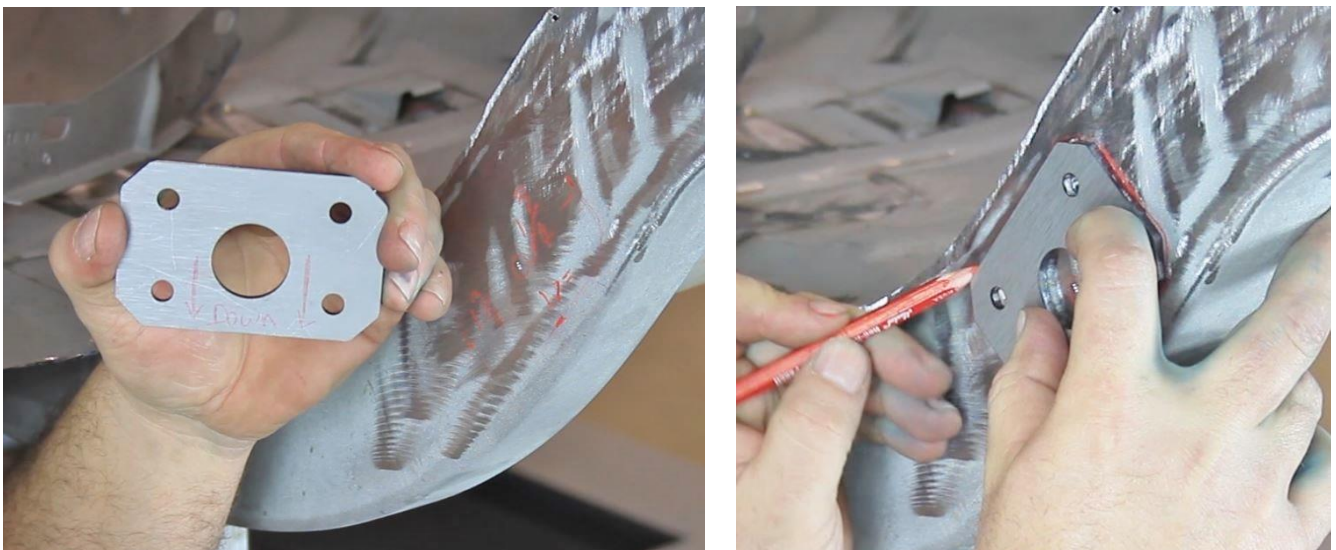
Figure 16 – Upper Link Mount Frame Rail Doubler
