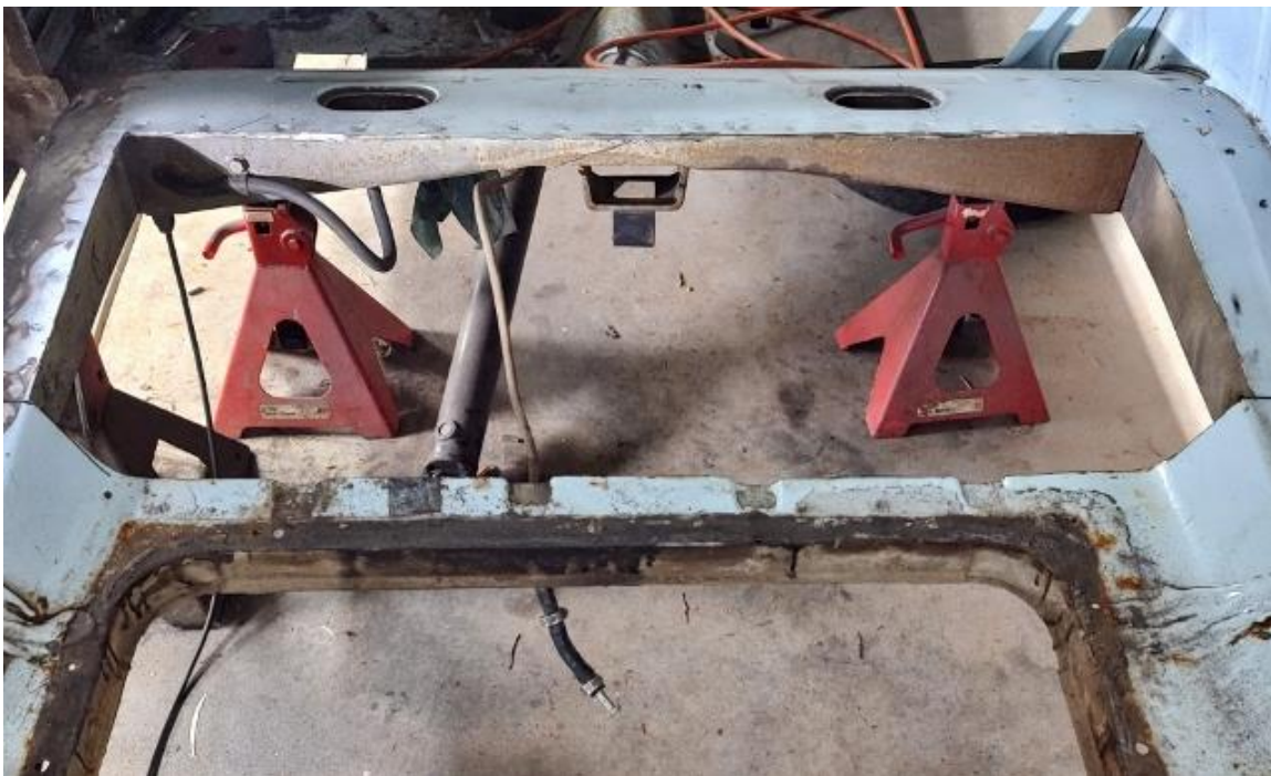
Figure 3 – Cut Trunk Floor
