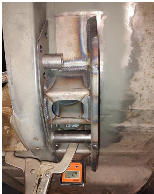
Figure 20 - Weld Torque Box
