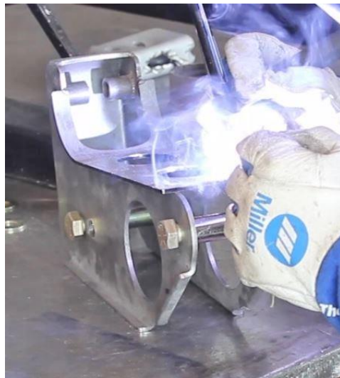
Figure 26 – Weld Axle Bracket Reinforcement
