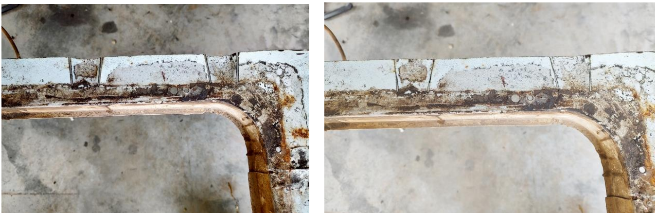
Figure 4 – Flatten Trunk Floor
