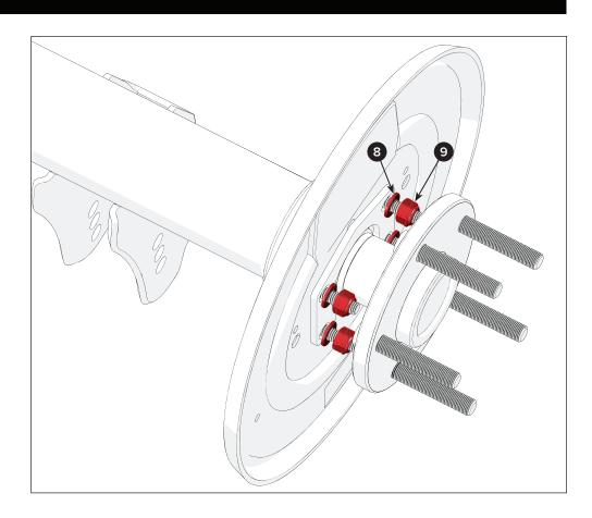
Use a torque wrench and socket to set the locknuts to 33 lb-ft (44.75 N-m). Use a crisscross pattern to spread the clamp load evenly.
