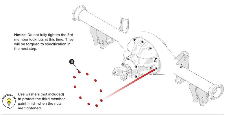
Attention: Due to the pinion yoke offset, two nuts can only be accessed with an open-end or crowfoot wrench. A crowfoot can be used with a torque wrench to set the correct torque settings.
