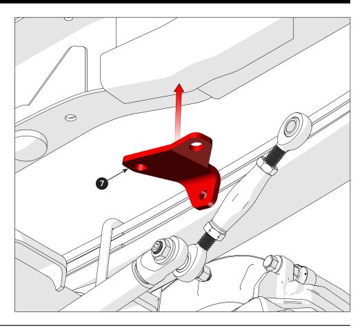
Then, align the mount bracket with the bend in the frame (B), as shown in the illustration.
