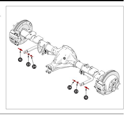
Install the sway bar links, assembled in step 6, onto the high alignment studs.
