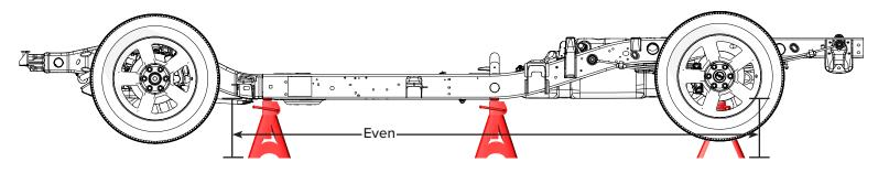
First, remove the lug nuts and wheels from both the left and right sides of the rear of the vehicle.
