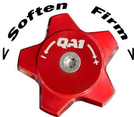
**SINGLE ADJUSTABLE**- Turn the adjustment knob counter-clockwise until the knob stops- This is the softest setting. Turn the knob clock-wise to firm the rebound.
