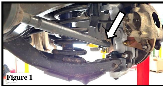
12. Slowly lower the jack supporting the lower control arm to release any remaining spring pressure. A spring compressor may need to be used to safely release all pressure.
