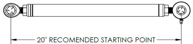
17. Install bushing end of trailing arm into third hole from the top of the notch bracket using 9/16" x 3.5 hardware in the Trailing Arm Hardware Kit (p/n 7039-230). **(Figure 8)** Final torque of 85 lb. ft. should be applied only with the truck at final ride height. Changing the instant center by raising or lowering the trailing arm on this bracket should be parallel to the ground can be adjusted after final ride height is determined.
