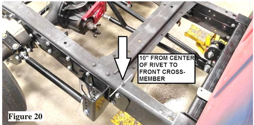
33. 10" from the center of the frame rivet is a starting position for the front cross-member. Before drilling and mounting the cross-member, slide cross-member until the torque arms front connection is vertical. **(Figure 21)** Once the connection is vertical, torque the cross-member to frame bracket hardware, then drill the frame for cross-member mounting holes and torque all 7/16" x 1.25" hardware to 49 lb. ft.
