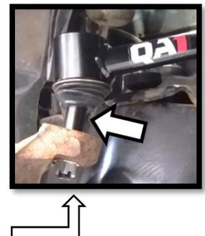
24. The included steering rack is an OE type '79-'93 mustang (Cardone P/N 97-207). Attach steering rack to lower cross-member using 5/8" x 5.5" bolts (#20), one .120" thick washer (#19) under bolt head, with 5/8" SAE washers (#22) and nylock nut (#23). **(Figure 25)**
