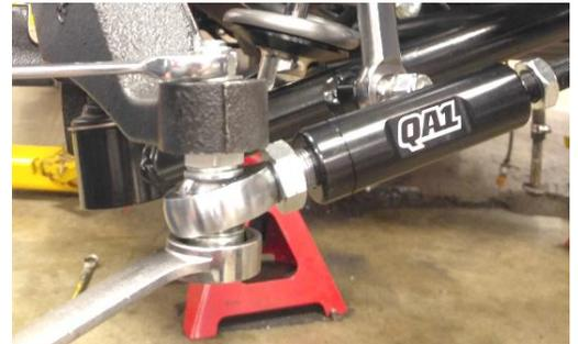
26. Install the left hand threaded 5/8" jam nut (#15) onto left hand threaded 5/8" rod end (#14). Thread the tie rod sleeves onto rod end until threads bottom out. **(Figure 26)**
