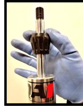
19. Install the coil-overs with the adjustment knob(s) towards the top, facing outward. **(Figure 24)**
