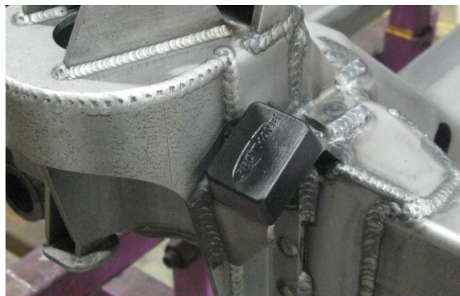
Figure 6 - Installed UCA Bump Stop
