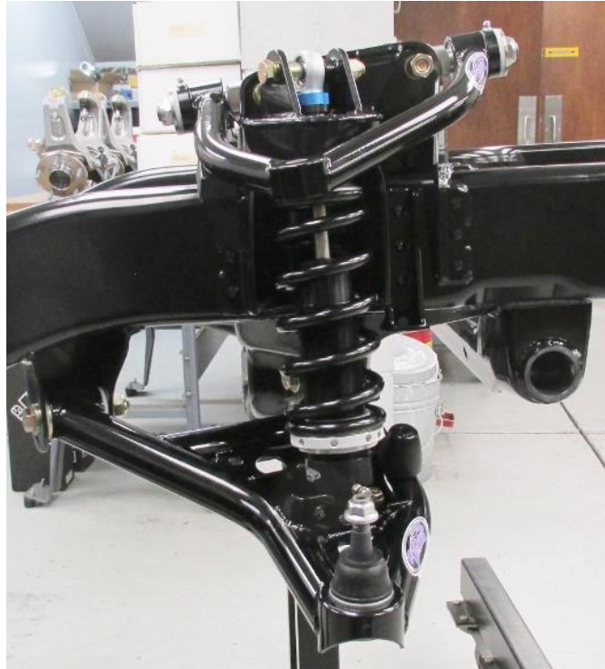
Figure 10 - Installed Coilover View
