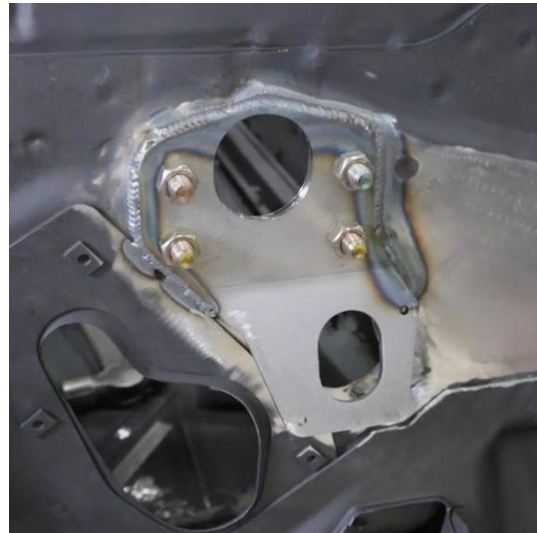
Figure 7 - Weld Bracket to Firewall
