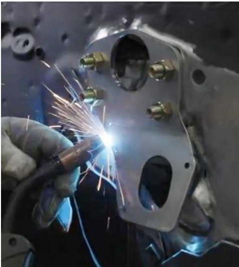
Figure 7 - Weld Bracket to Firewall
