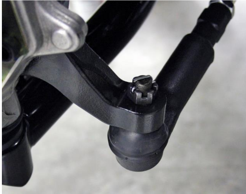
Figure 21 – Install Tie Rod Ends to Steering Arms
