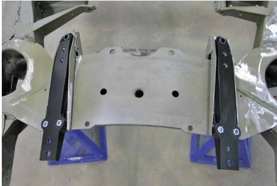
Figure 6 - Install Adapter Plates to Crossmember
