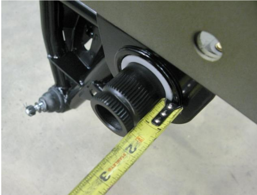
Figure 17 – Install Splined Sway Bar
