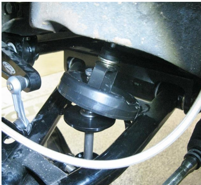
Figure 28 - Install Coilover Shock Assembly
