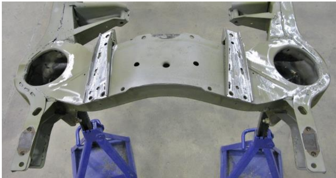
Figure 3 - Grind Lower Control Arm brackets
