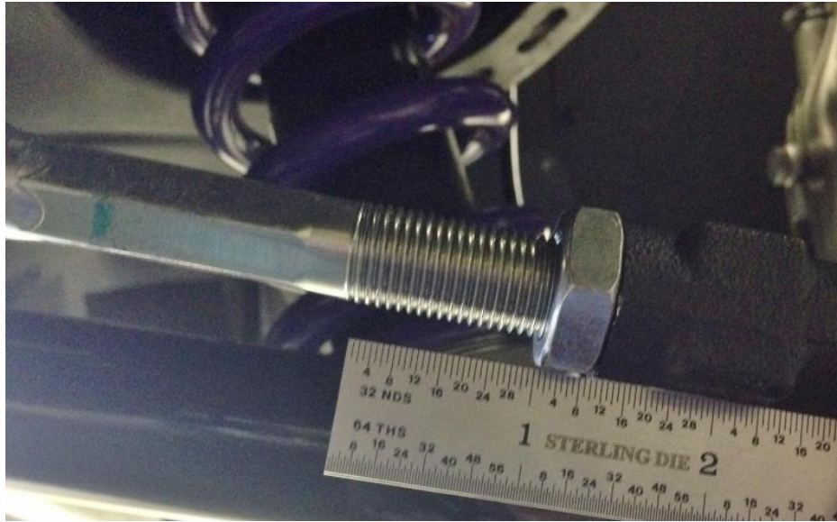
Figure 11 - Install the Tie Rod Ends
