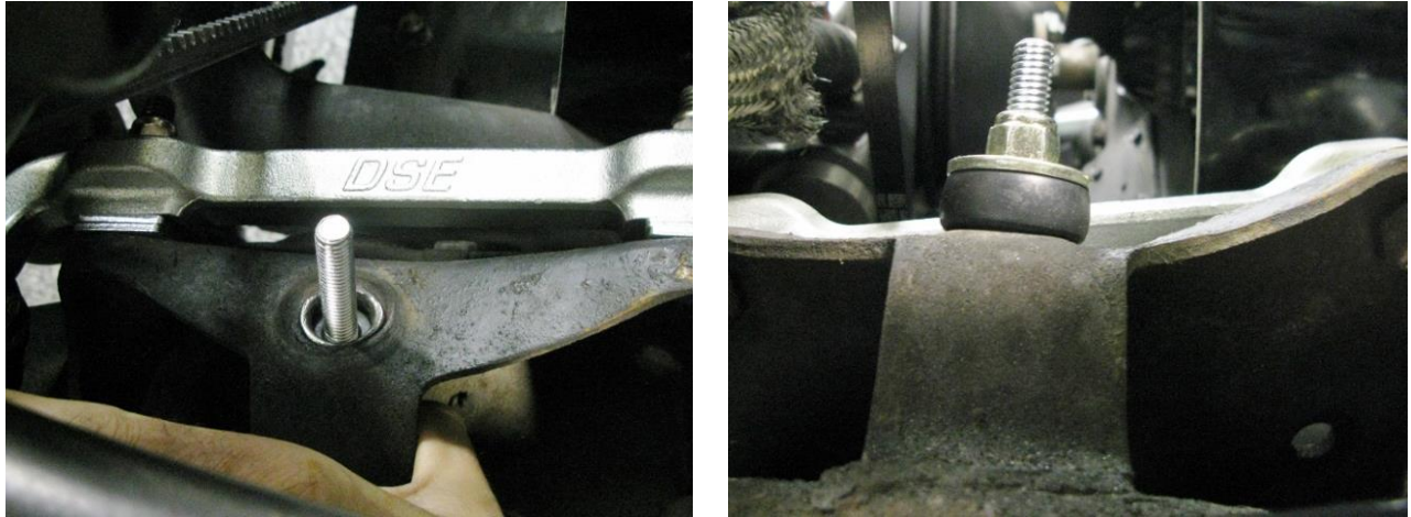
Figure 29 - Tighten Coilover Upper Mount Assembly.
