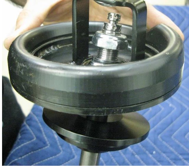
Figure 27 - Assemble Coilover Upper Mount
