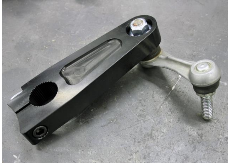
Figure 19 – Install Endlinks to the Sway Bar Arms
