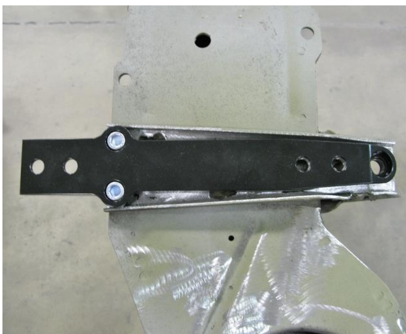
Figure 4 - Position Cradle Crossmember Adapter Plates
