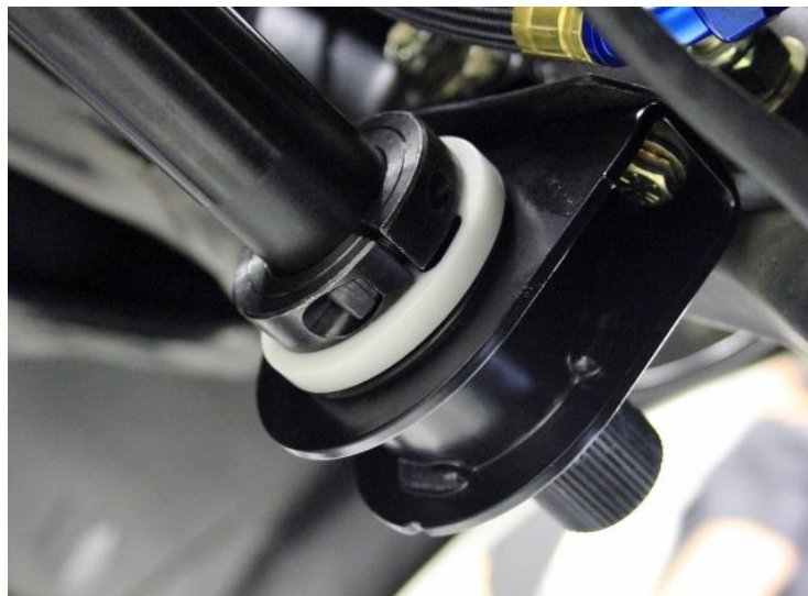
Figure 18 – Install Sway Bar Split Lock Collars
