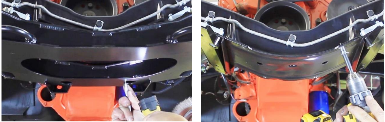
Figure 7 - Locate & Drill Mounting Holes
