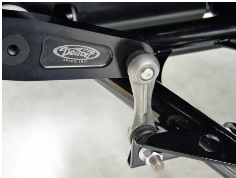
Figure 22 – Install the Sway Bar End Links to the Lower Control Arms
