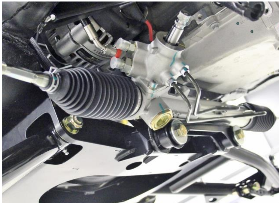
Figure 12 - Install Rack & Pinion
