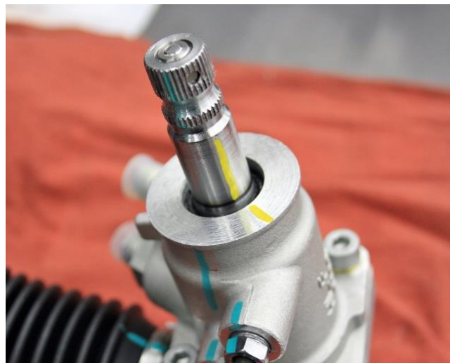
Figure 10 - Center the Rack and Pinion
