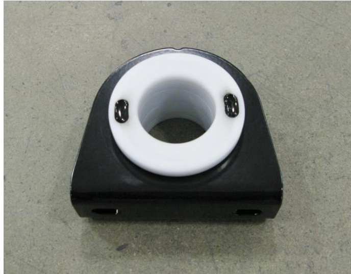
Figure 15 – Install Sway Bar Composite Bushings
