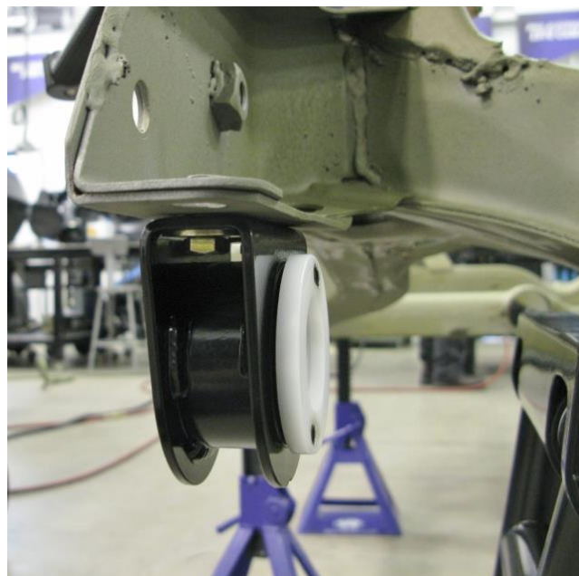
Figure 16 – Install Sway Bar Bracket Assembly
