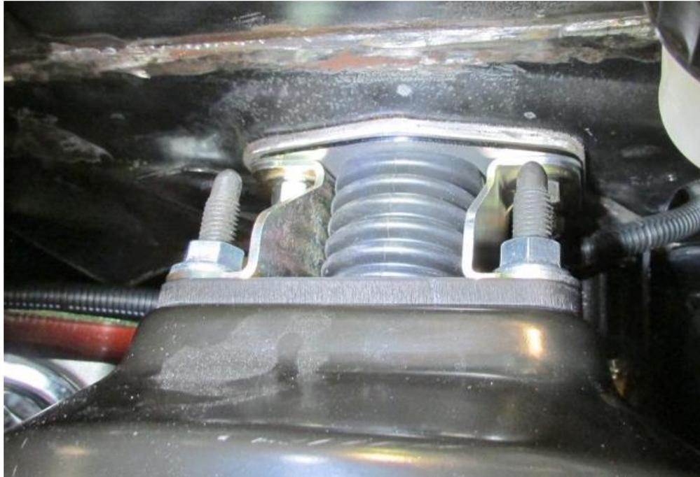
Figure 1 - Install Brake Booster/Master Cylinder to Firewall
