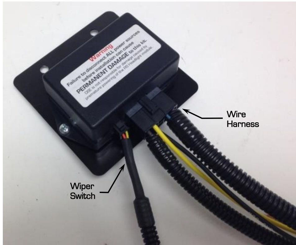
Figure 26– Connect Wiper Switch & Harness to Module
