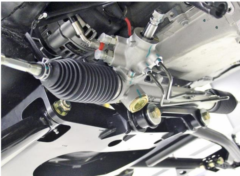
Figure 23 – Install Rack & Pinion
