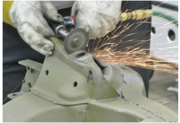
Figure 5 – Cut Factory Upper Shock Mount
