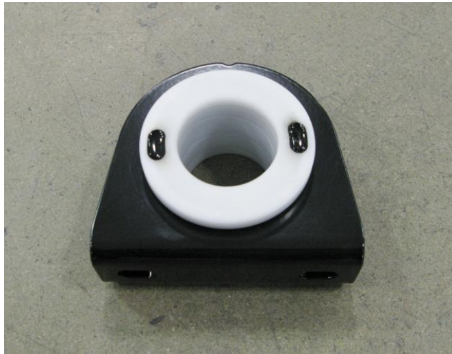
Figure 26 – Install Sway Bar Composite Bushings
