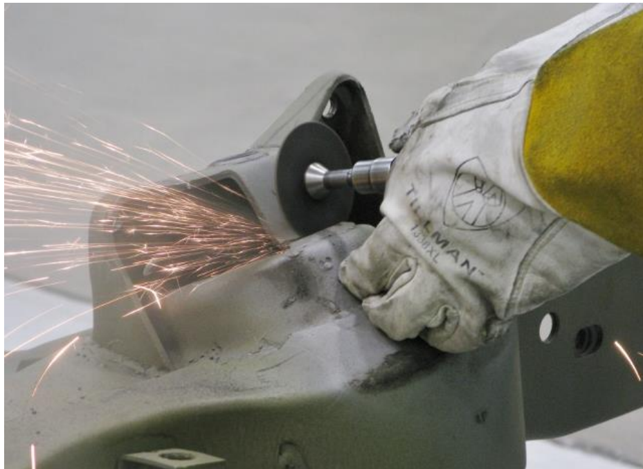
Figure 6 – Cut Factory Upper Shock Mount Bracket
