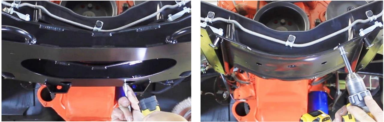
Figure 18 - Locate & Drill Mounting Holes
