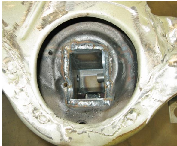
Figure 12 - Weld the Bottom of the Coilover Pocket to the Spring Perch
