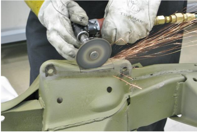
Figure 5 – Cut Factory Upper Shock Mount
