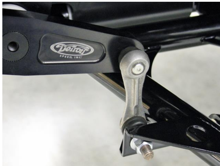
Figure 33 - Install the Sway Bar Endlinks to the Lower Control Arms
