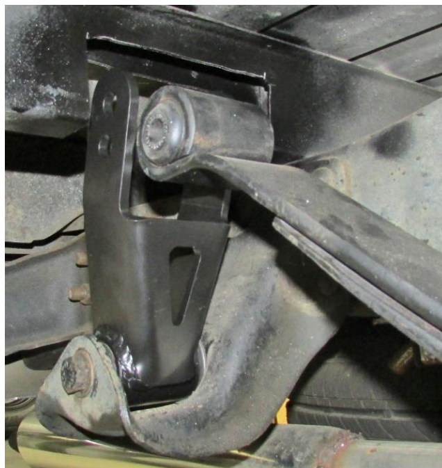
Figure 2 - Install Drop Shackle
