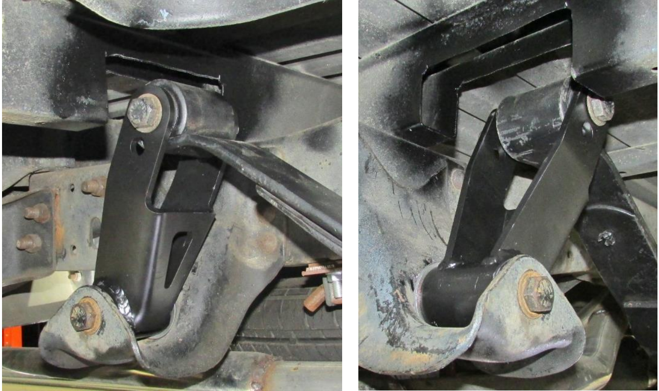
Figure 3 – Install Leaf Spring
