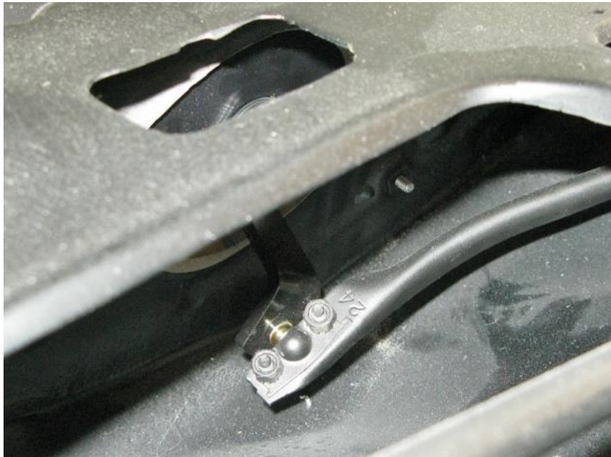
Figure 3 - Attach Pitman Arm to Wiper Linkage
