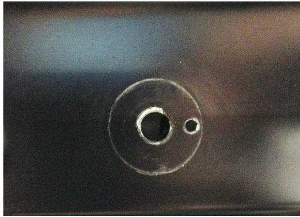
Figure 5 - Drill Anti-Rotation Hole
