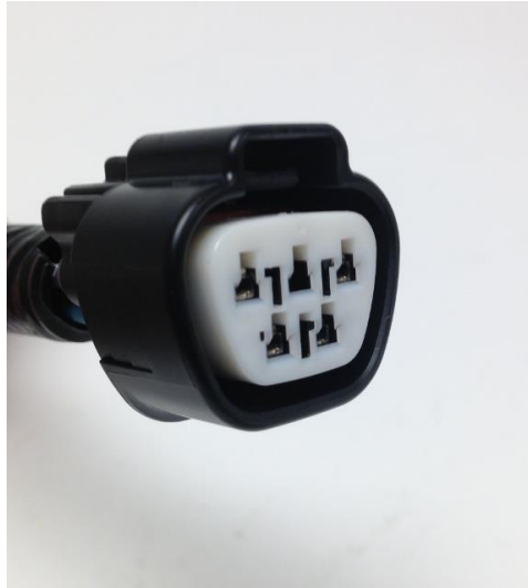
Figure 9 - Wiper Motor Connector
