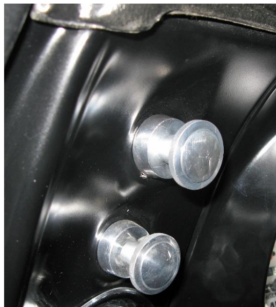
Figure 8 - 1967 Camaro Switch/Knob Installation
