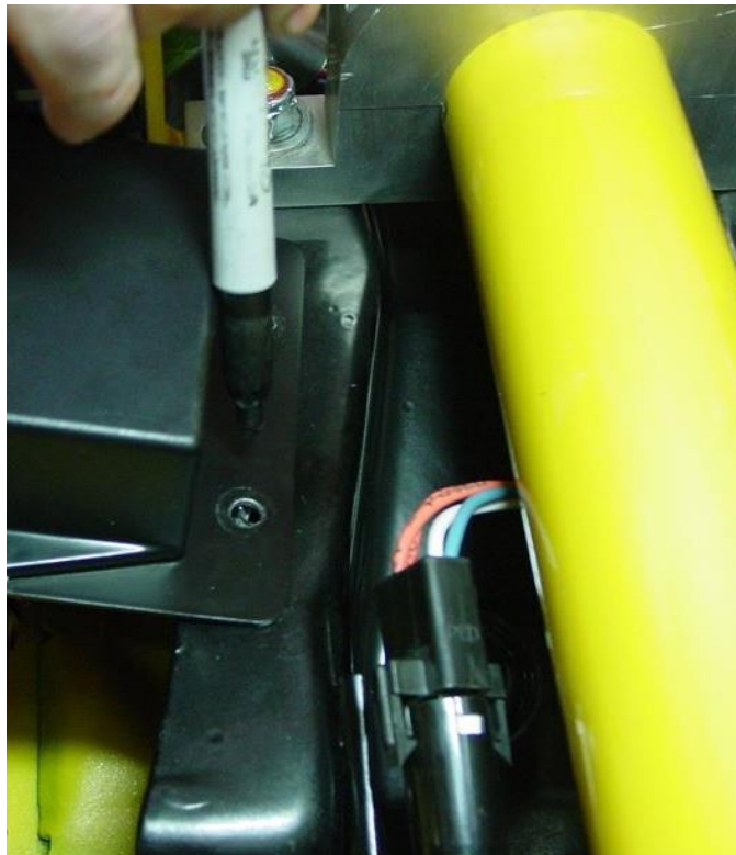
Figure 12 – Locate the Bolt Holes
