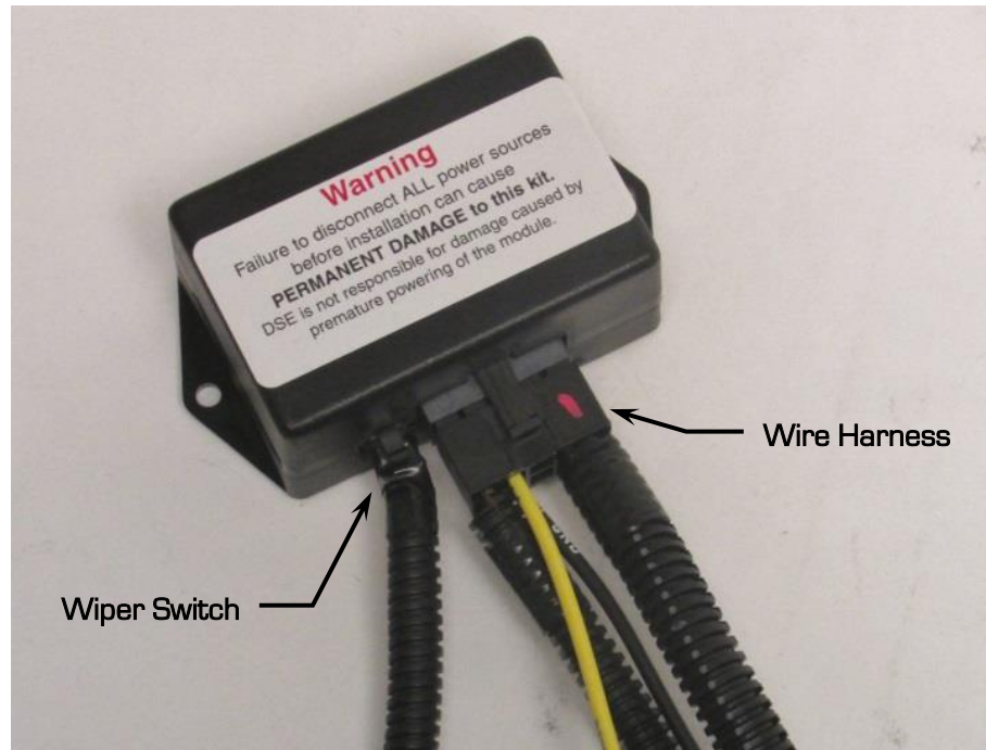
Figure 15 – Connect Wiper Switch & Harness to Module
