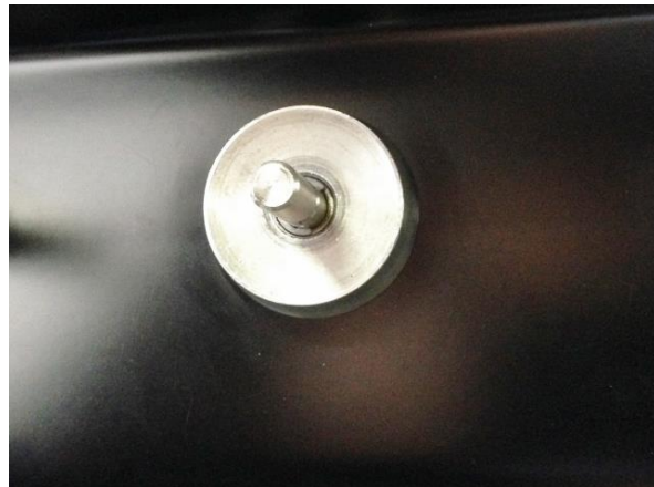
Figure 7 - Thread Bezel onto Switch
