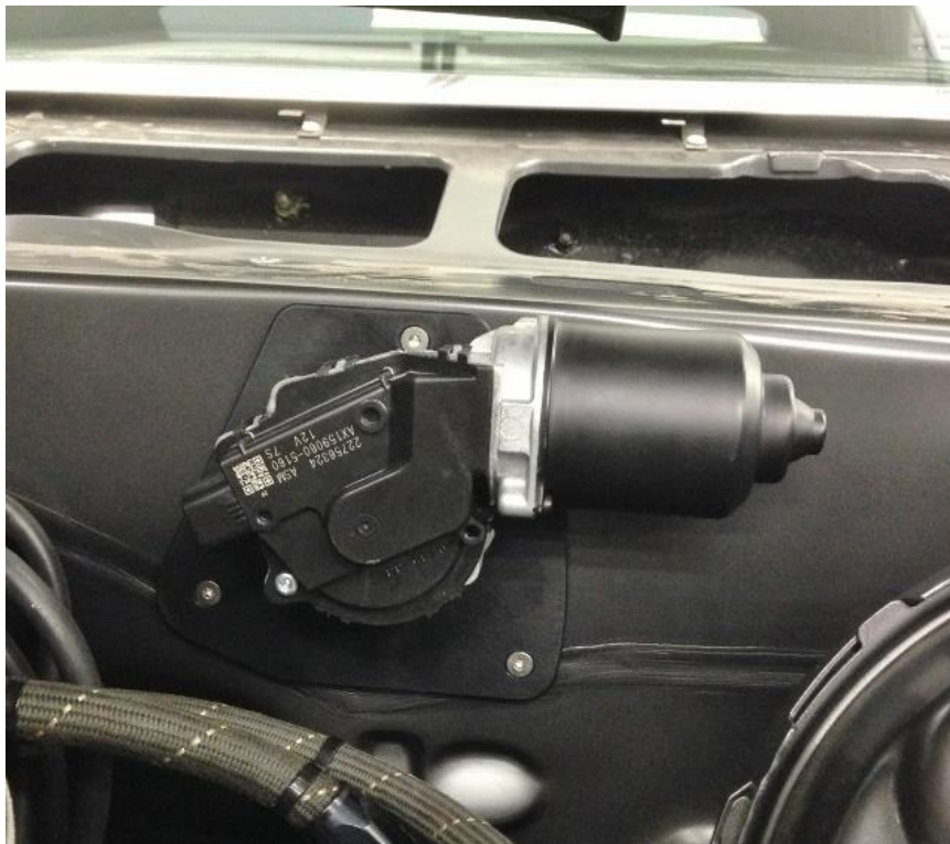
Figure 1 – Attach Wiper Motor to Firewall
