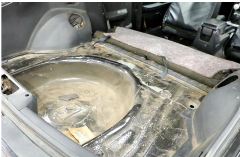
Figure 4 - Remove Trunk Carpet
