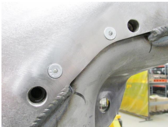
Figure 8 – Countersink Nut Plate Holes
