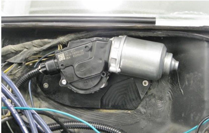
Figure 7 – Install Wiper Motor Connector
