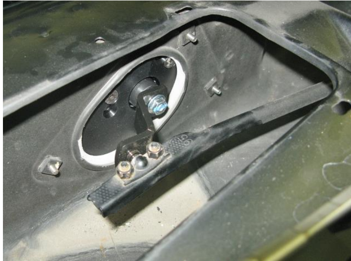
Figure 11 – Attach Pitman Arm to Wiper Linkage
