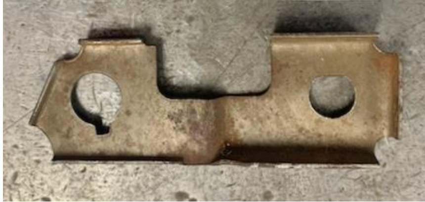
Figure 4 - Remove Factory Switch Bracket
