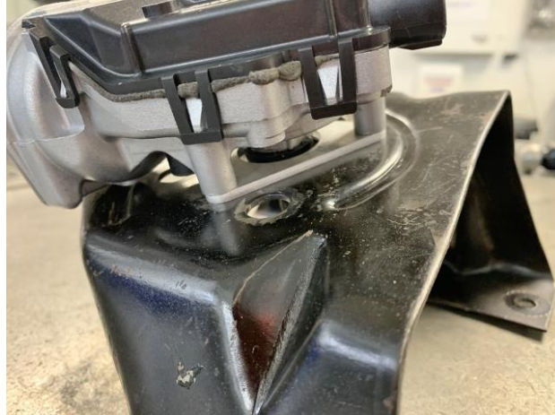
Figure 14 - Drill Motor Mount Holes
