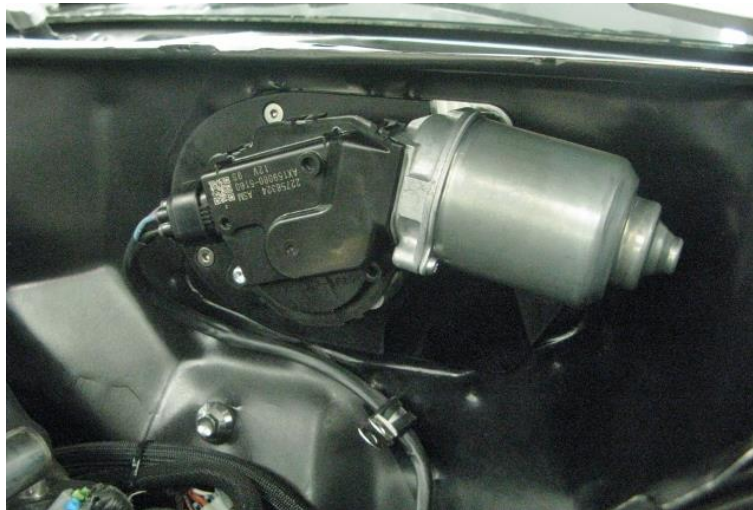
Figure 7 - Install Wiper Motor Connector
