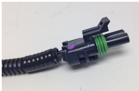
Figure 8 - Washer Pump Connection
