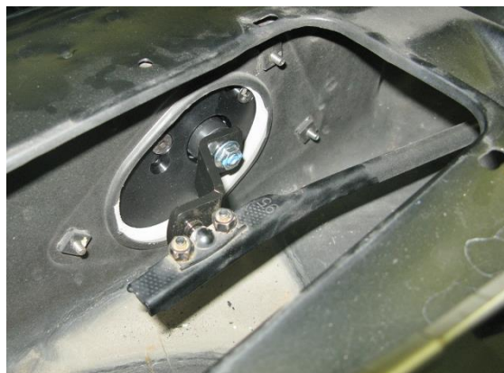
Figure 3 - Attach Pitman Arm to Wiper Linkage
