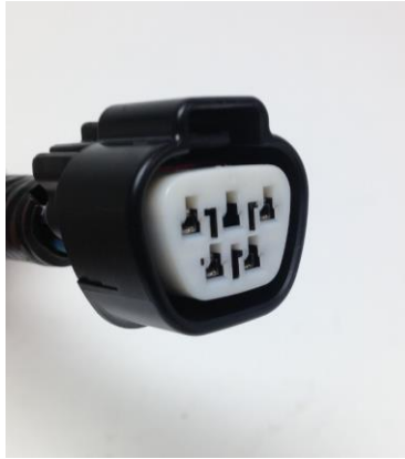
Figure 6 - Wiper Motor Connector
