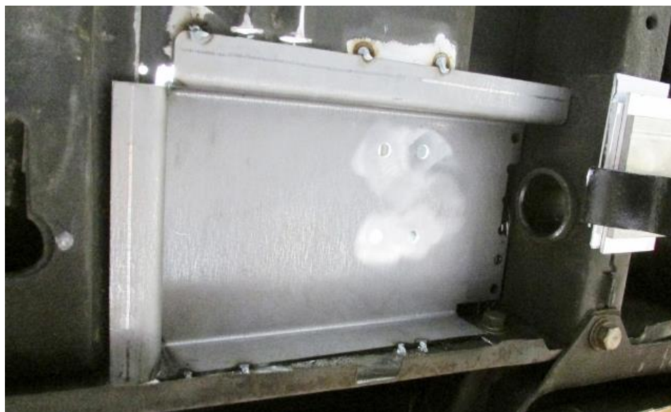
Figure 12 - Tack Weld Rear Mount
