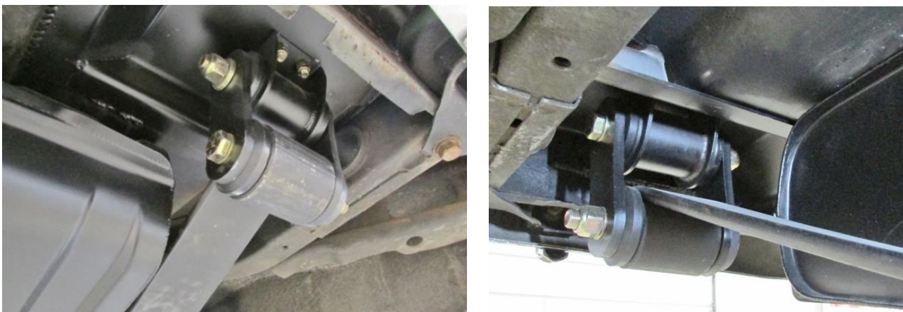
Figure 19 - Install Rear of Leaf Spring
