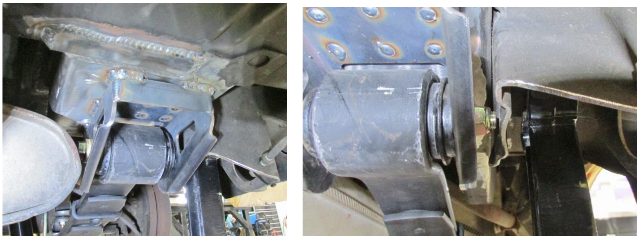
Figure 18 - Install Front of Leaf Spring
