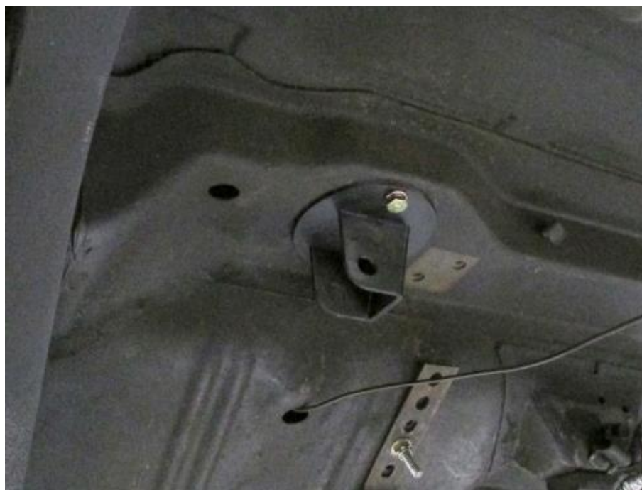
Figure 17 - Install Shock Assembly (Driver Side)
