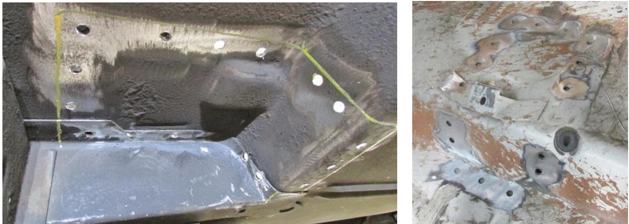
Figure 8 - Drill Plug Weld Holes
