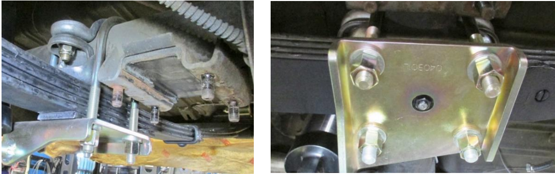
Figure 20 – Install Lower Shock Plates
