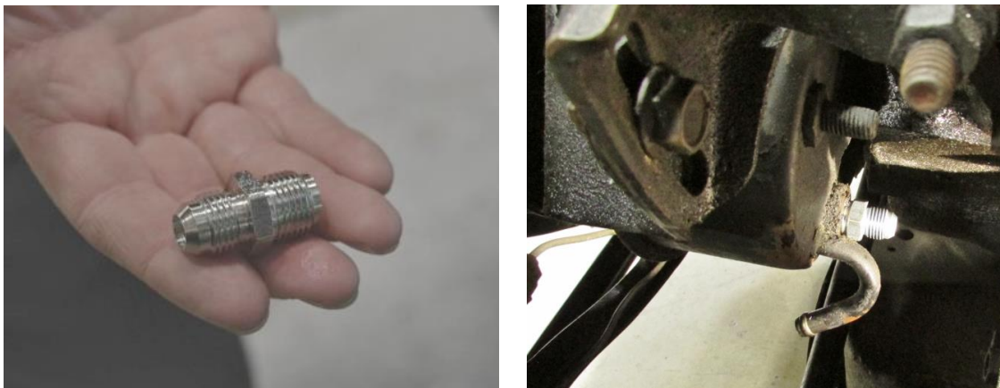
Figure 7 - Install P/S Pump Fitting
