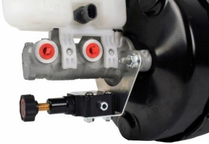
Figure 1 - Completed Bracket Installation
