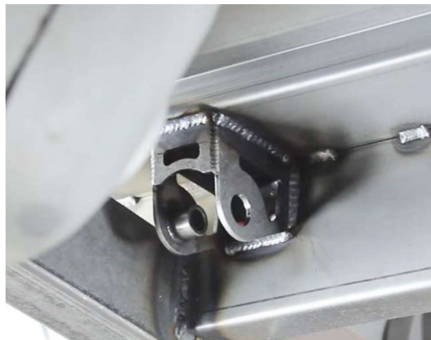
Figure 24 - Weld Upper Shock Mounts
