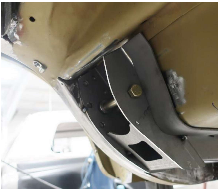
Figure 13 - Tack Weld Upper Link Pocket
