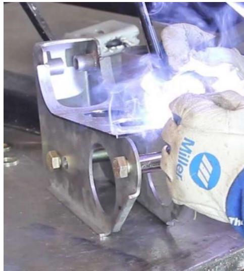
Figure 30 - Weld Axle Bracket Reinforcement
