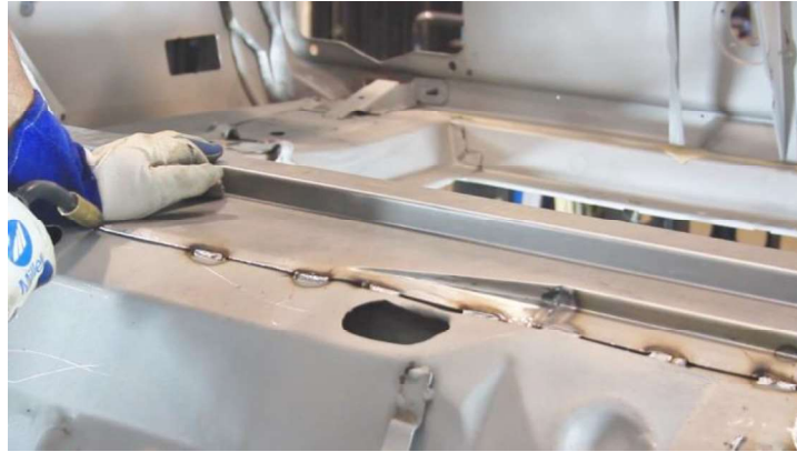
Figure 22 - Stitch Weld Front of Crossmember
