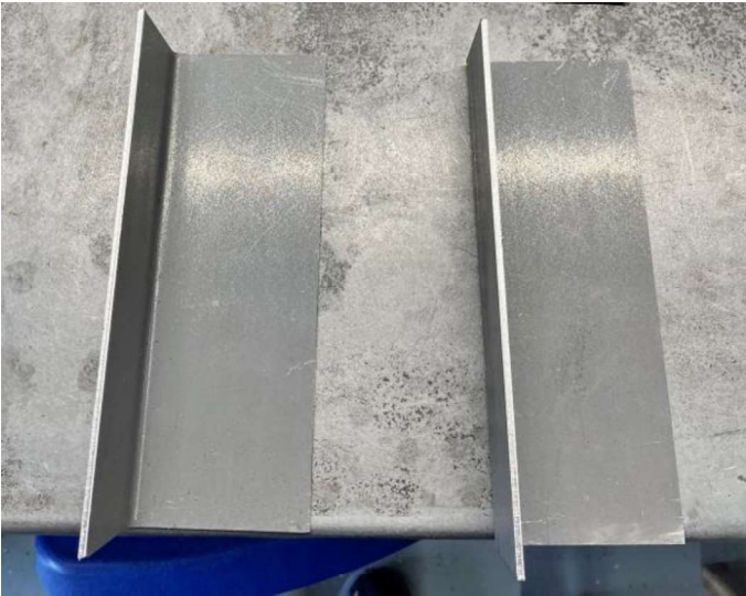
Figure 19 – Trim and Weld Closeouts
