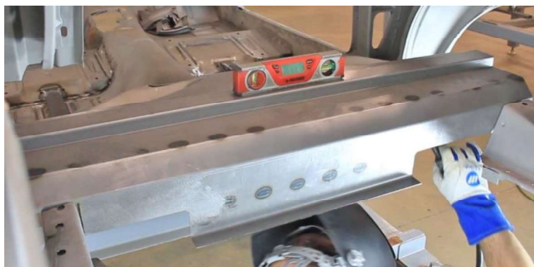
Figure 21 – Weld Upper Crossmember
