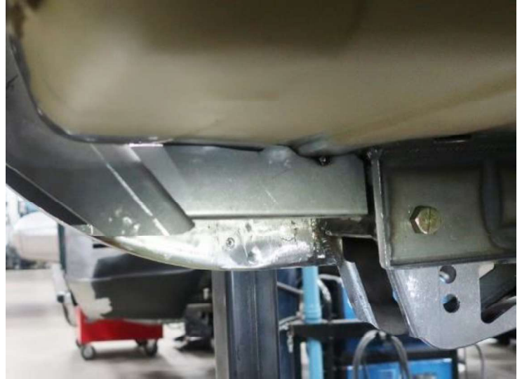
Figure 19 – Trim and Weld Closeouts
