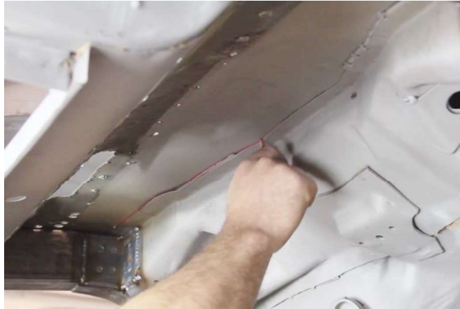
Figure 1 - Mark Floor Pan Cut Line (Underneath Vehicle)
