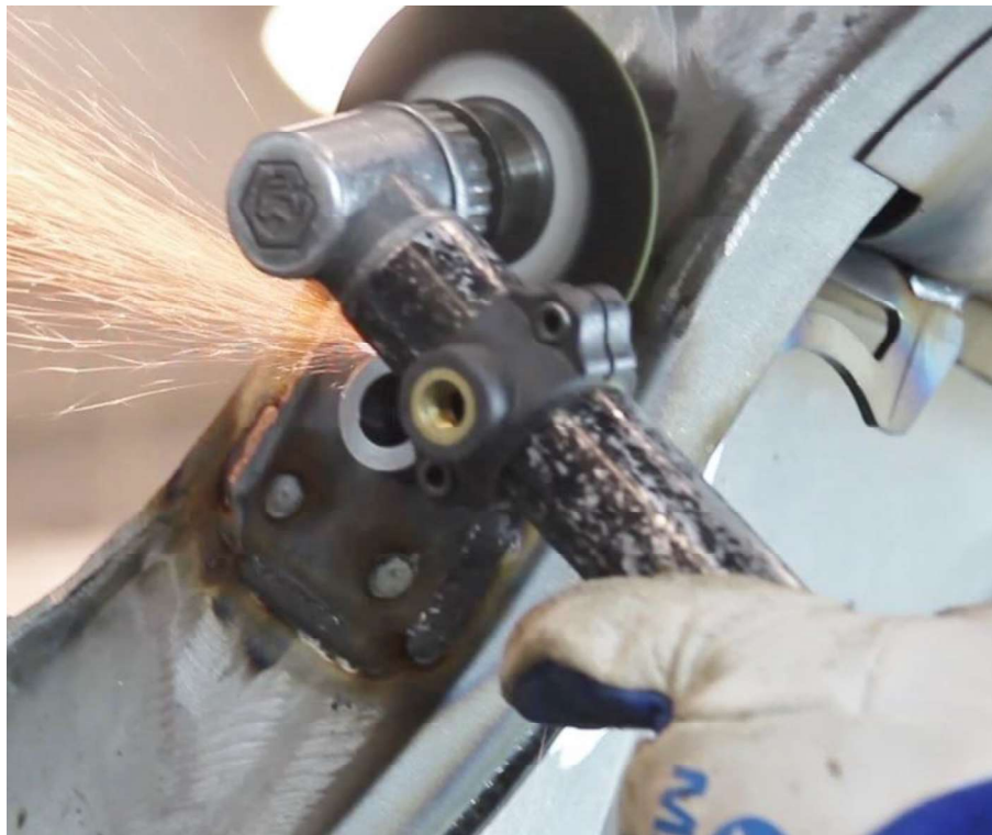
Figure 15 - Cut-Off Crush Tube Flush with Frame Rail
