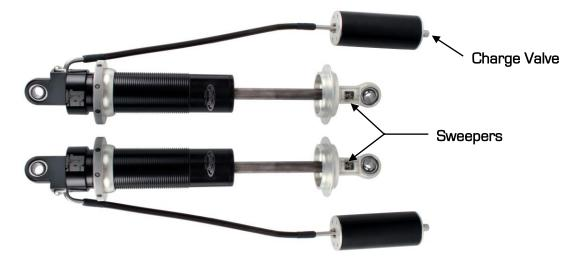
Figure 12a - Detroit Speed Double Adjustable Shock w/ Remote Canister
