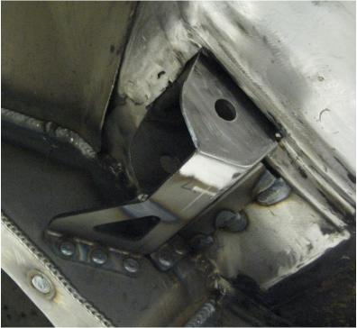
Figure 4 - Reinforcement Brackets
