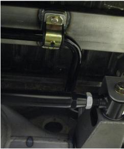
Figure 8 – ARB Spacer and Bracket
