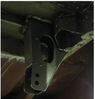
Figure 7 – Body Side Track Bar Bracket Page 7 of 15
