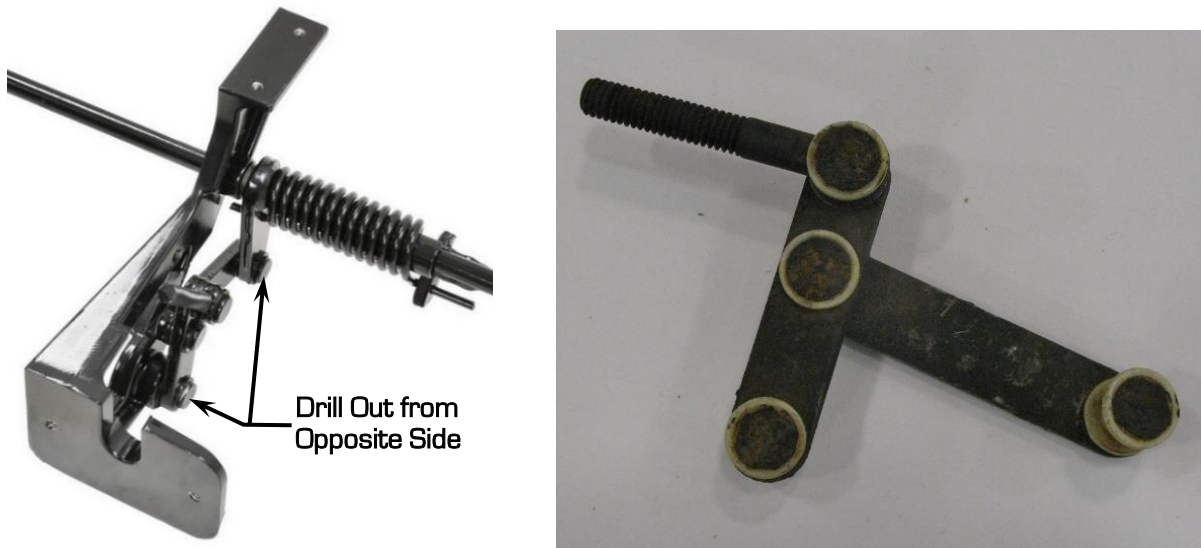
Figure 29 - Remove Factory Linkage
