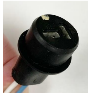
Figure 43 - Wrong Wire Position
