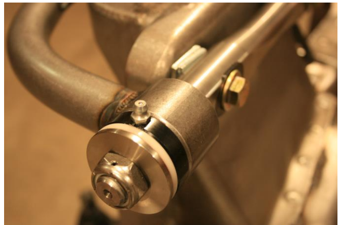
Figure 16 – Installed Upper Control Arm
