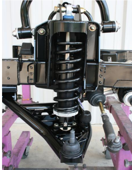
Figure 14 – Installed Coilover View
