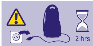
**WARNING:** The appliance should be UNPLUGGED, OFF and COLD before cleaning the appliance. Switch off and unplug the appliance from the outlet. Allow your appliance to cool down for at least 2 hours. It is preferable to clean the appliance BEFORE use.
