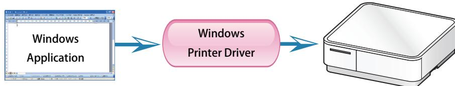
Install the mPOP Printer Software, and then connect a printer with a USB interface to the PC. The Plug and Play feature will enable the Windows printer driver automatically.
