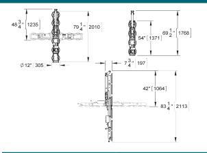
With a dual vacuum system, 1100 lbs [500 kg] load capacity, removable pad frame extensions and a remarkably low profile, this Powr-Grip® rotator/tilter provides maximum versatility and ease of use in tight work locations.
