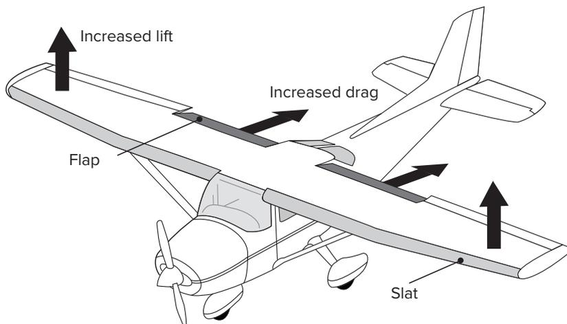
**Figure 1-15.** The location and function of flaps.
