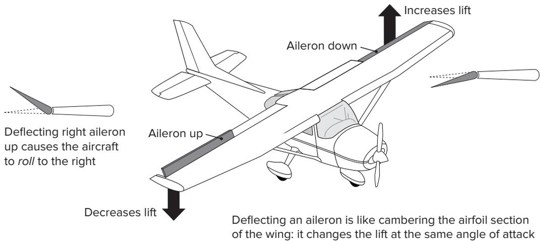
**Figure 1-14.** The location and operation of the ailerons.
