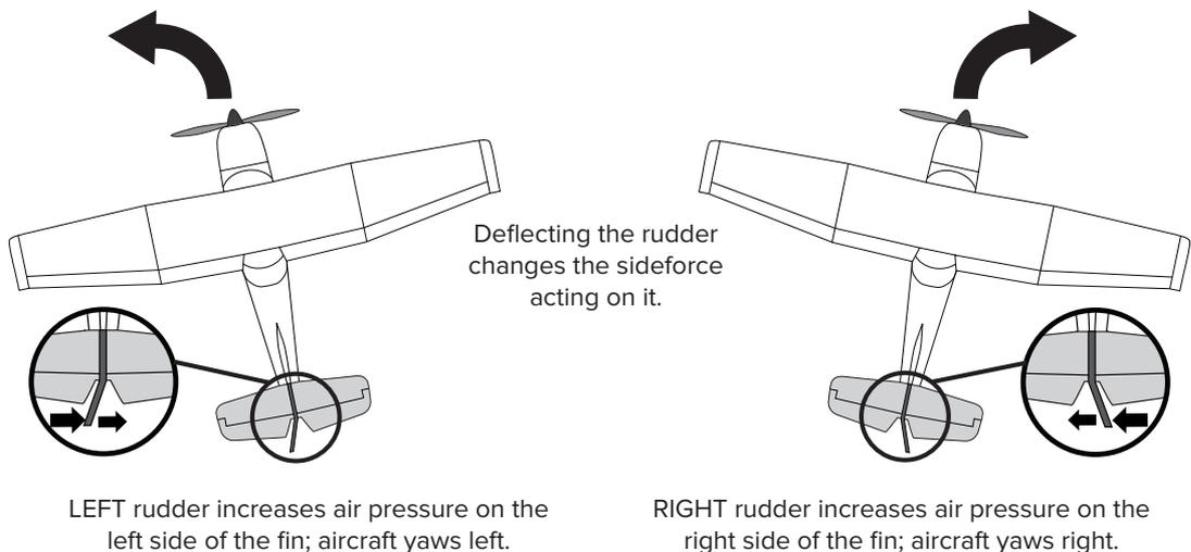
**Figure 1-13.** The location and operation of the rudder.
