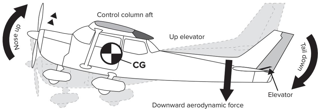
**Figure 1-12.** The location and operation of the elevator.
