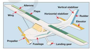
Figure 4-7. Parts of a small aircraft.
