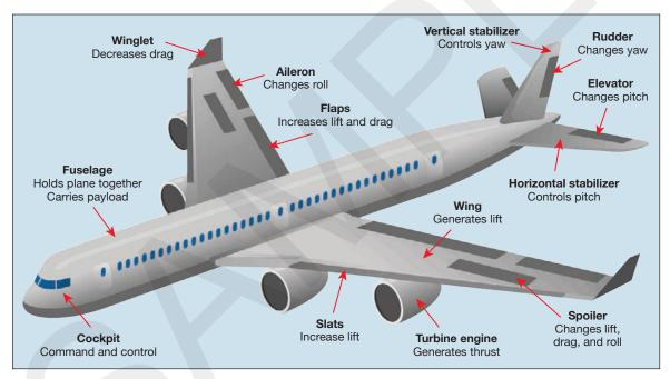
Figure 4-6. Parts of a large aircraft.
