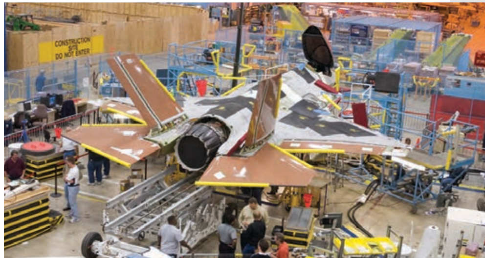
FIGURE 1-4. The F-35 Lightning II Joint Strike Fighter features vertical tail feathers and horizontal stabilators made from carbon fiber-reinforced bismaleimide composite. (Photo courtesy of Lockheed Martin)
