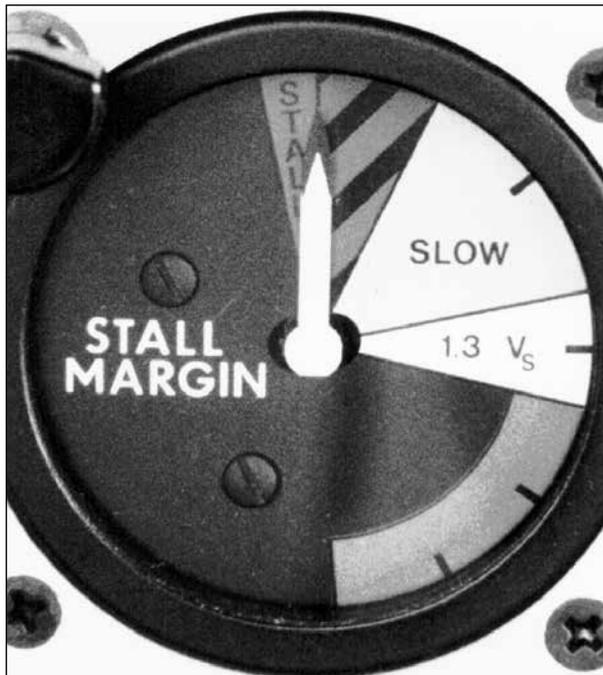
Figure 1-4. Angle of attack indicator
