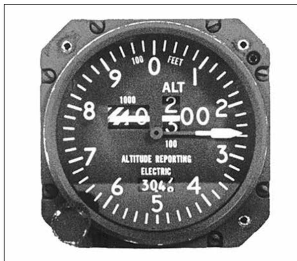
Figure 1-8. Drum-pointer altimeter
