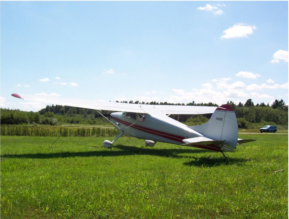
**Figure 1-3.** Taildraggers are fun to fly but should be approached with caution by pilots trained in tricycle gear aircraft.
