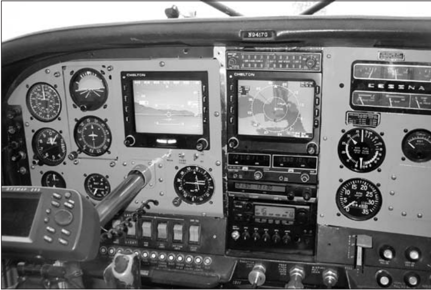
Figure 1-3. The Chelton Flight System, introduced in Alaska in 1999, was an immediate success in reducing accidents. (Courtesy of Chelton Flight Systems)
