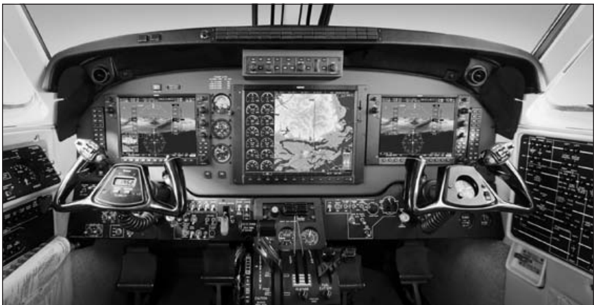
Figure 1-2. The Garmin G-1000 EFIS cockpit displays a multitude of information. (Courtesy of Garmin International)
