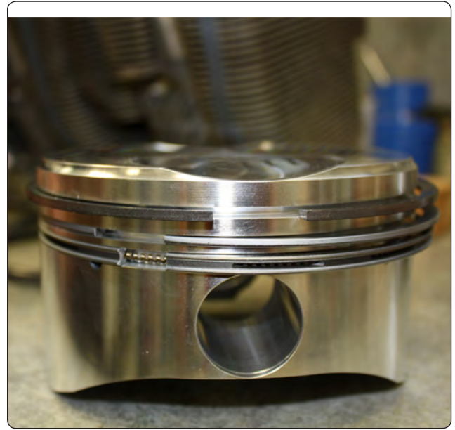
Figure 1-15. Machined rings around a piston.
