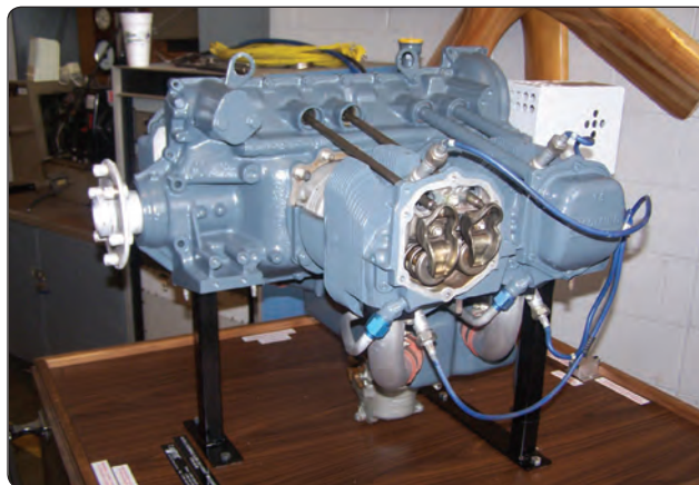
Figure 1-1. A typical four-cylinder opposed engine.
