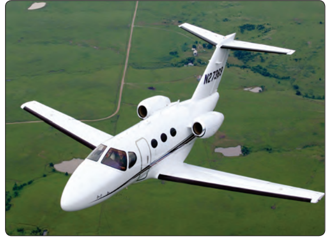
Figure 1-10. The nearly all composite Cessna Citation Mustang very light jet (VLJ).
