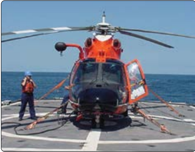
Figure 1-13. Example of mooring of a helicopter.
