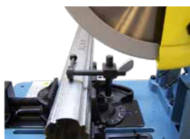
Excentric clamping system
