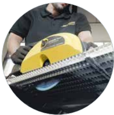
Ideal for cutting metal sheets, gratings and sandwich panels up to 2 5/8" (67 mm)
