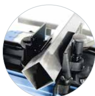
„K“ CLAMPING SET FOR SQUARE TUBES
