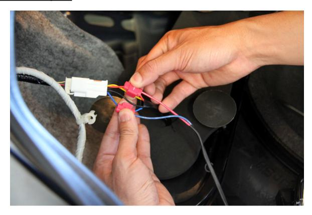
Once you've installed the bumper light in place on the rear bumper, you will thusly need to connect the red and blue wire to the wiring from the lower bumper light. The blue wire will be connected to the blue/silver wire as shown below. You might have to cut a little of the rubber sleeve on the bumper lights wiring to give yourself a little more space. Again, if you do not want the flashing feature, you WILL NOT connect the red wire.
