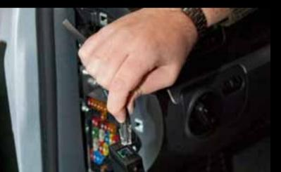
Pull the entire cable through the fuse box and snap the new vent into place starting at the top. Push on the bottom corners of the vent to firmly secure into place.
