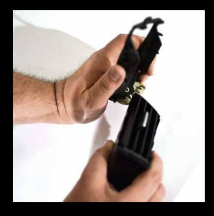
Pull down and forward until the bottom clips release and the entire front cover of the vent will come off.
