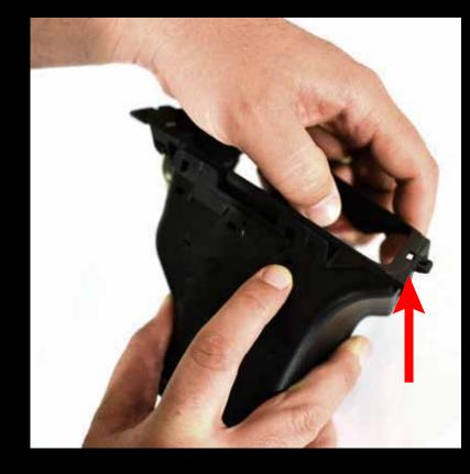
Unclip the front clip on the right side of the vent and flex the front of the vent forward.
