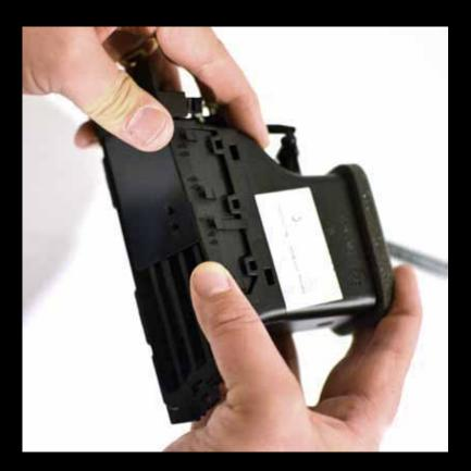
Re-attach the vent face. BOTTOM FIRST, after clipping the bottom side, then clip in the top.
