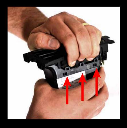
Unclip the 3 top clips of the vent as shown. You can simply put pressure between the clips and pull forward.
